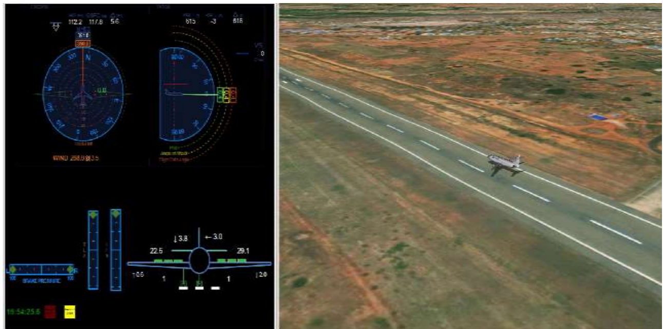
Figure 15: Deployment of reversers, brakes and speed brakes
