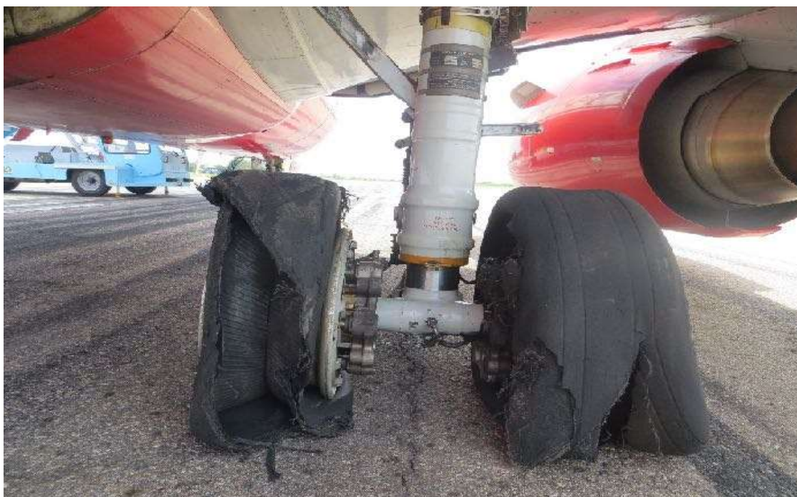
Figure 9: Failed Tyres No. 3 and No. 4
