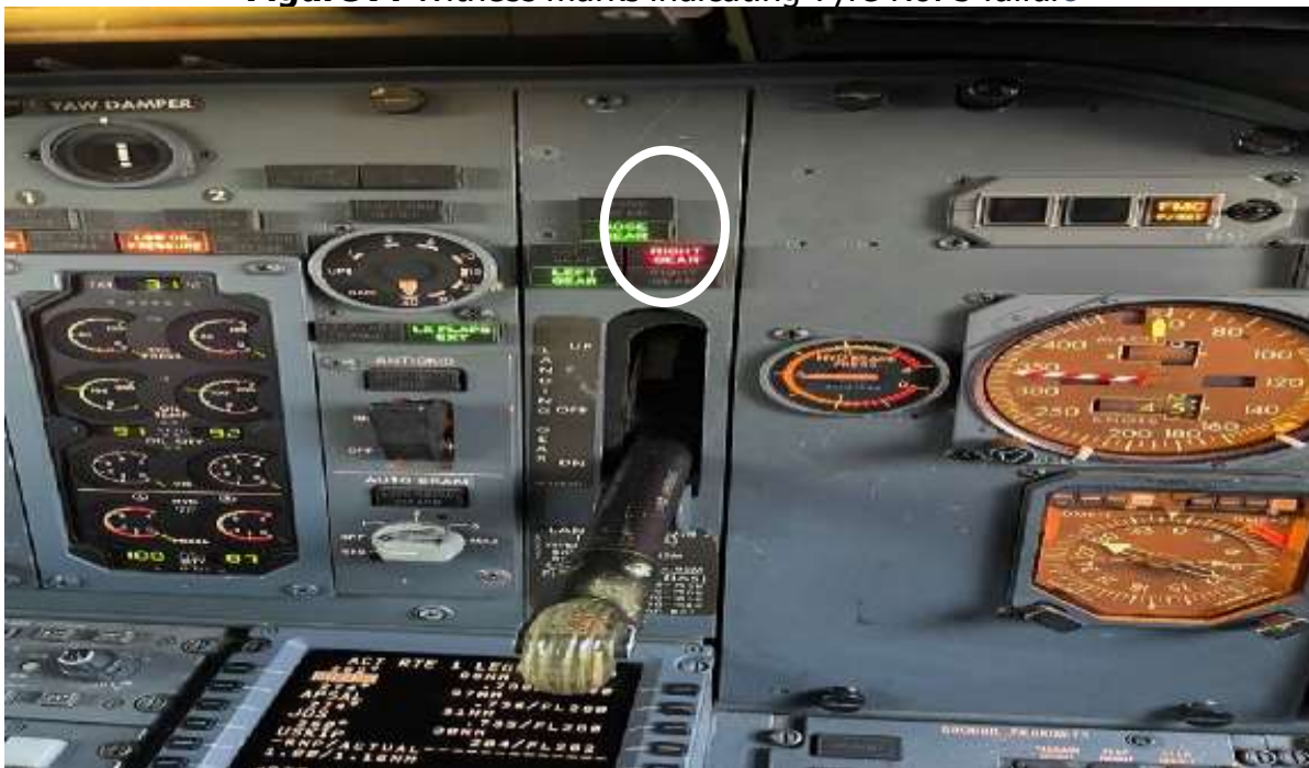
Figure 8: Landing gear indications in the cockpit
