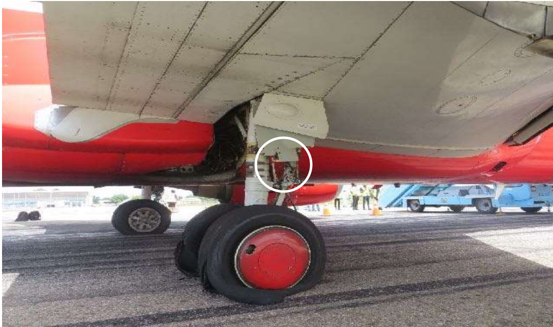
Figure 11: Torn section of Right MLG shock strut door
