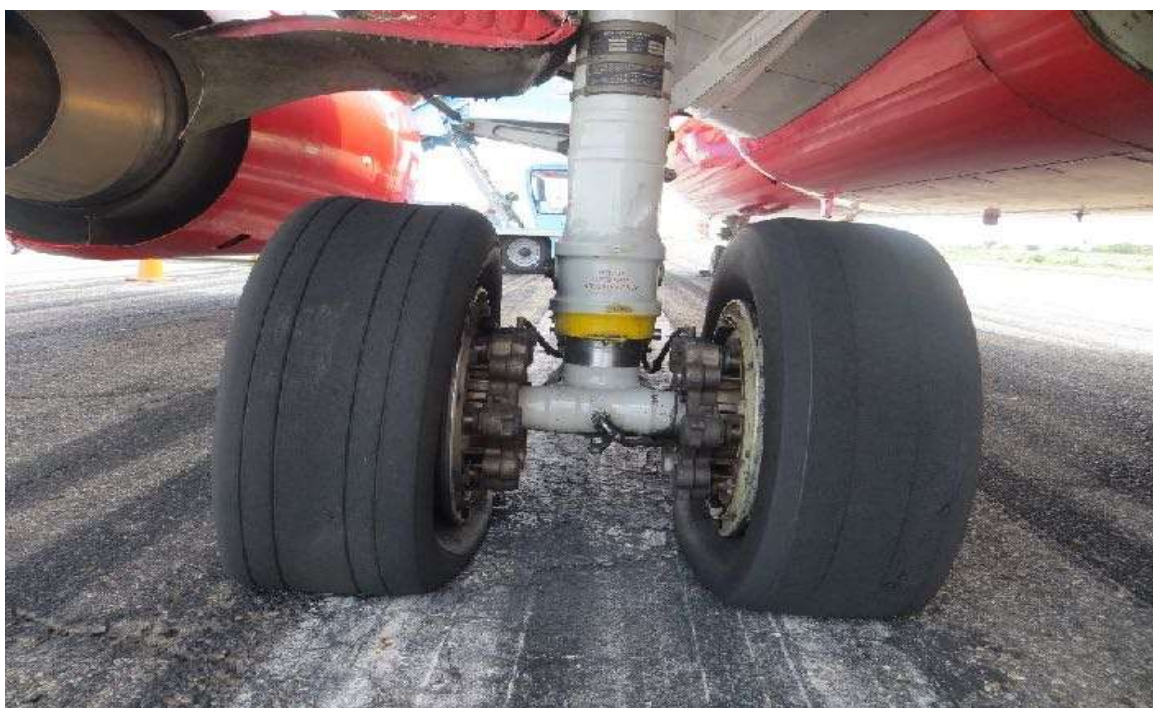
Figure 9: Failed Tyres No. 3 and No. 4
