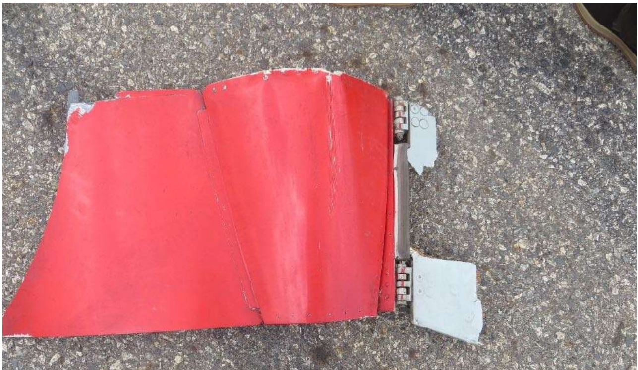
Figure 11: Torn section of Right MLG shock strut door
