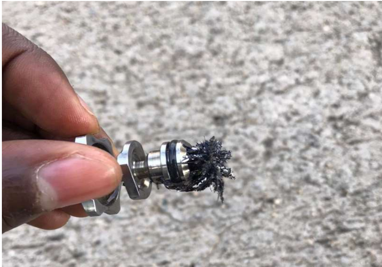
Figure 1: Magnetic Plug with chips
