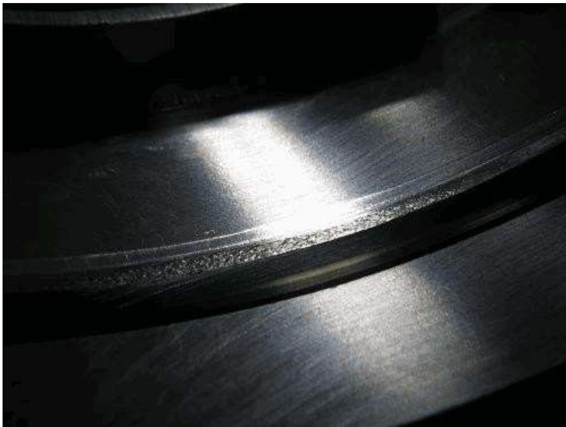
Fig 7: FRONT SUMP HOUSING (FRETTING) - DETAIL
