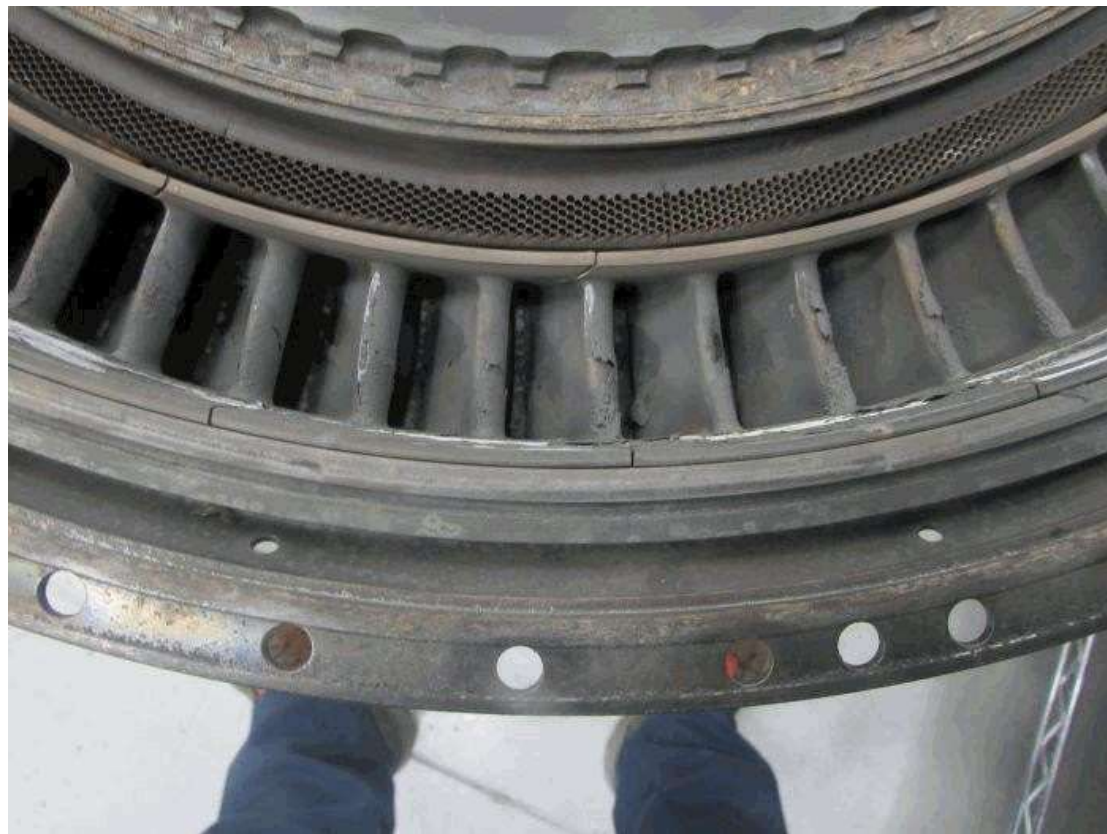
Fig 15: 2ND STAGE HIGH-PRESSURE TURBINE VANES - DETAIL
