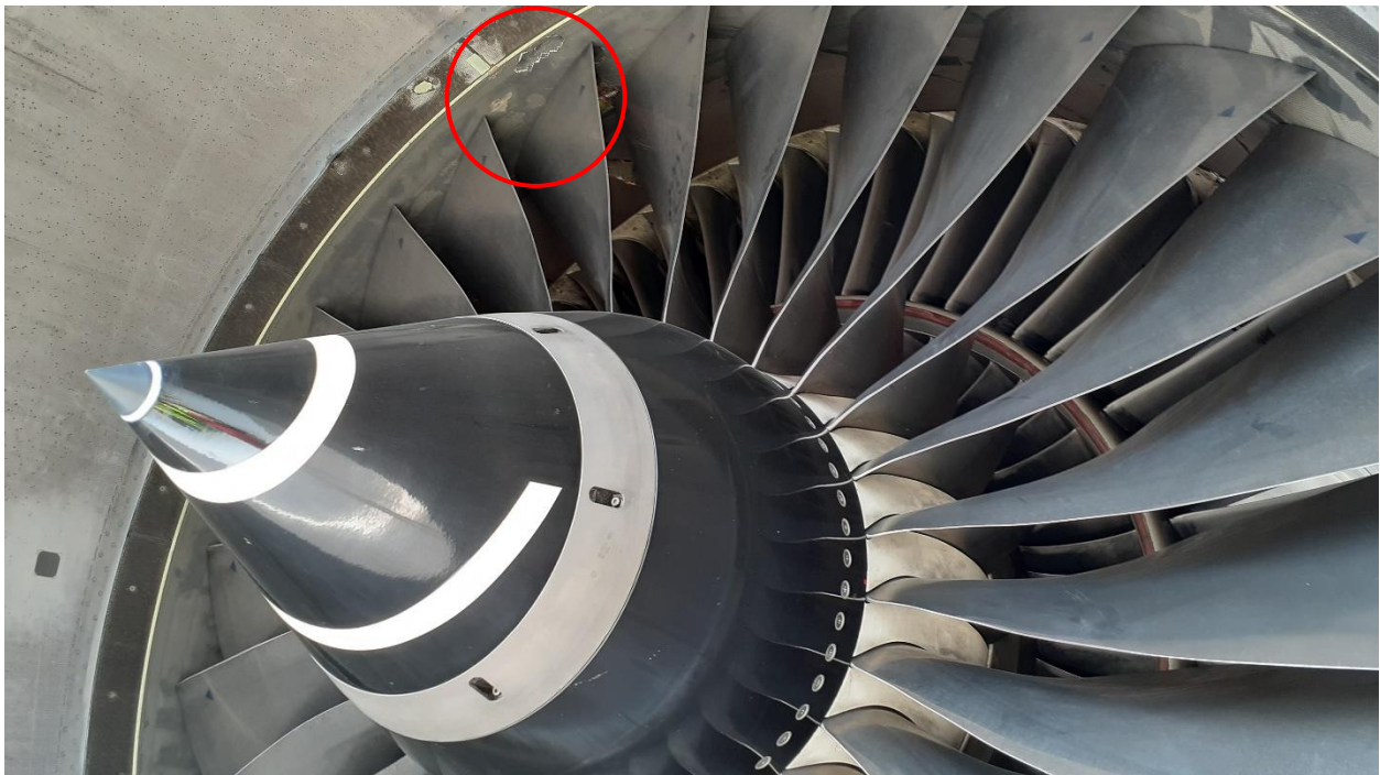
Figure 4: A close-up photo of the observed damaged area (circled)
