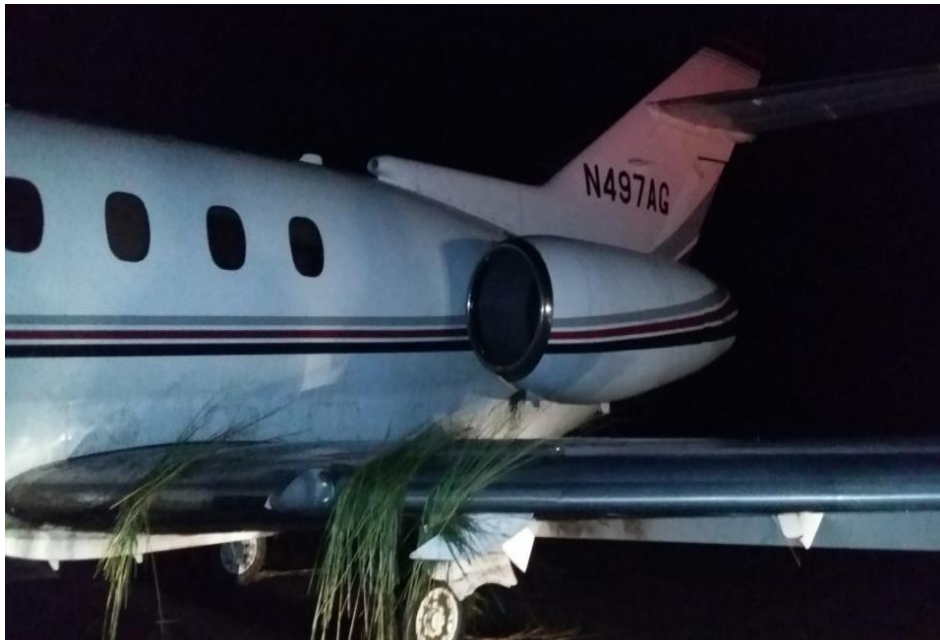
Figure 2: Photo of grass collection on the left wing and generator cooling inlet
