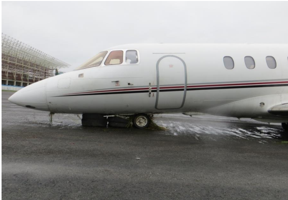
Figure 4: Photo of collapsed nose wheel landing gear
