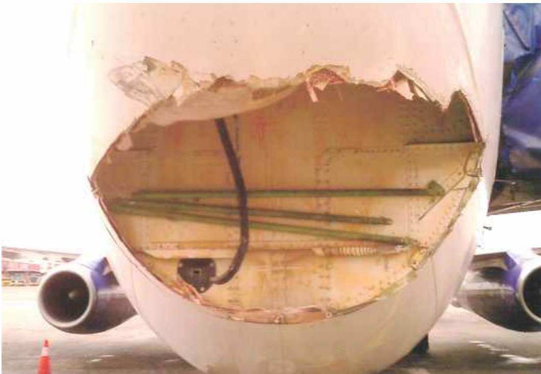
Fig.5 Exposed weather radar antenna at the lower part of the radome
