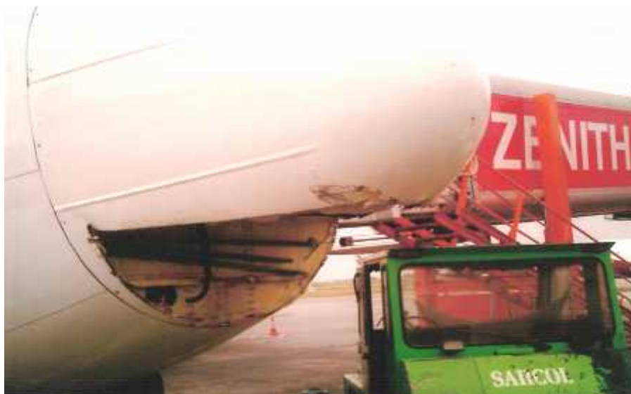
Fig.1 Tow tug damage to the lower Radome
