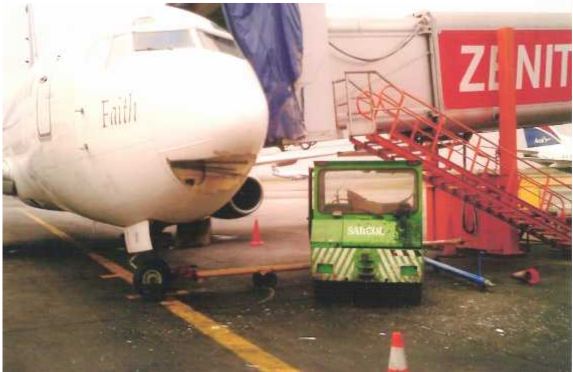
Fig.3 Nose gear turned beyond 90° exceeding the turning limit
