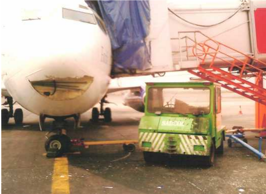
Fig.2 Exposed portion of the lower radome with the tow bar that turned the nose wheel beyond its limit
