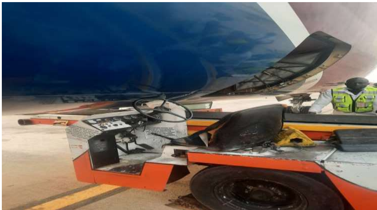
Figure 2: The conveyor belt truck still under the aircraft after the occurrence
