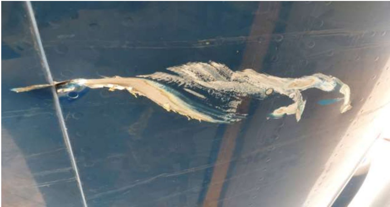
Figure 3: Puncture to the fuselage of the Arik air aircraft (a pressurised section of the aircraft)
