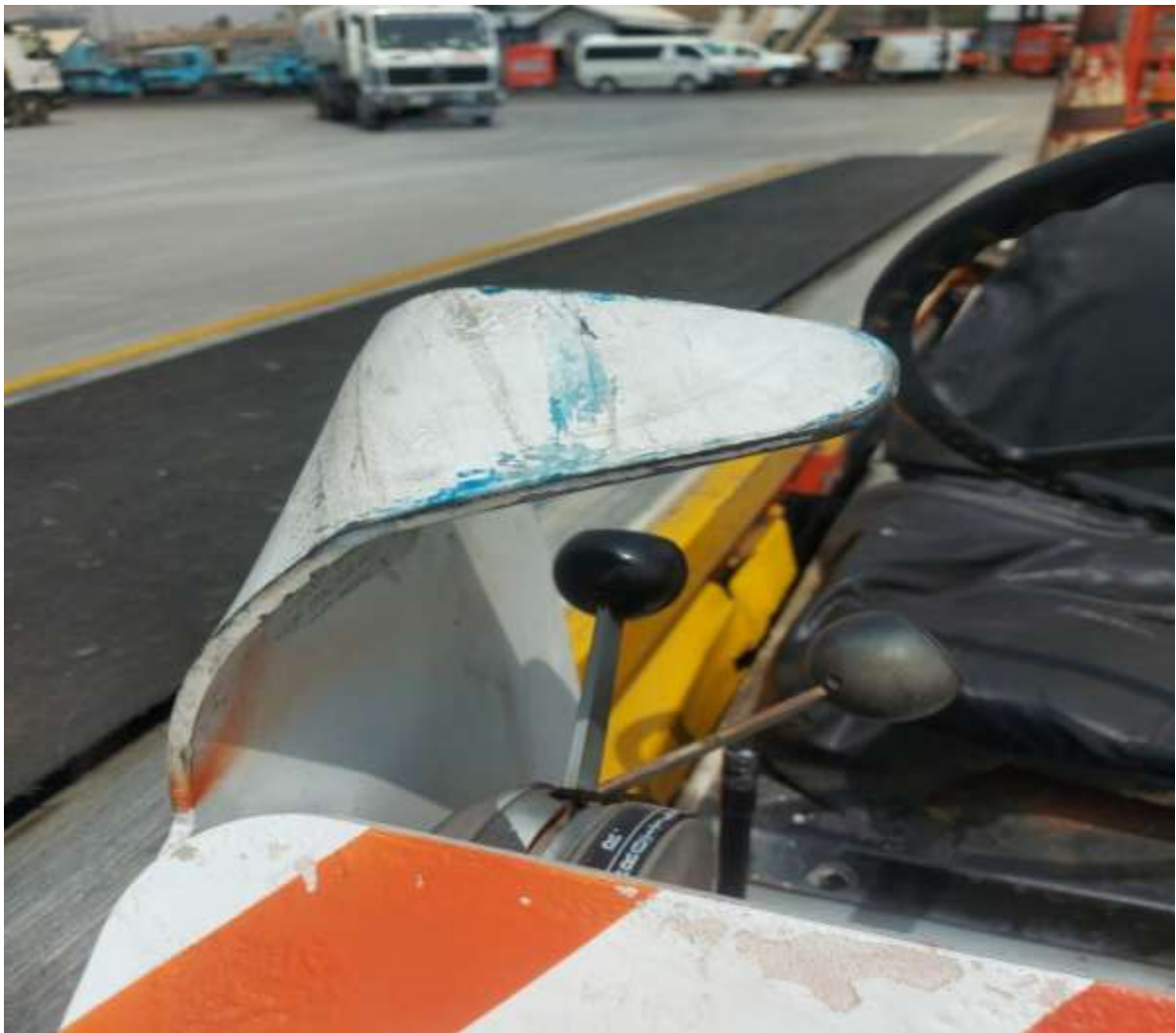
Figure 6: Head protector of the conveyor belt that punctured the fuselage of the aircraft
