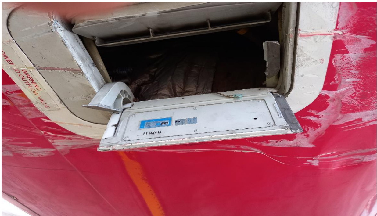
Figure 6: Broken outflow valve.
