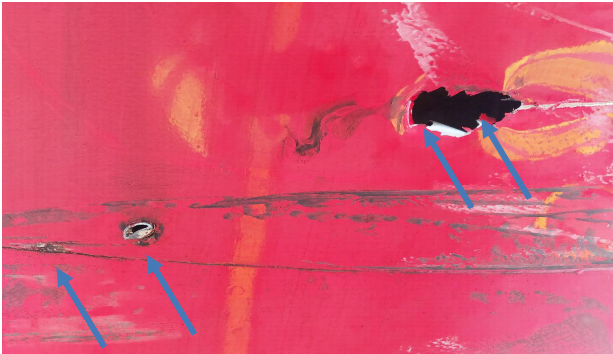
Figure 5: Three holes on the aft of the fuselage unpressurised area.
