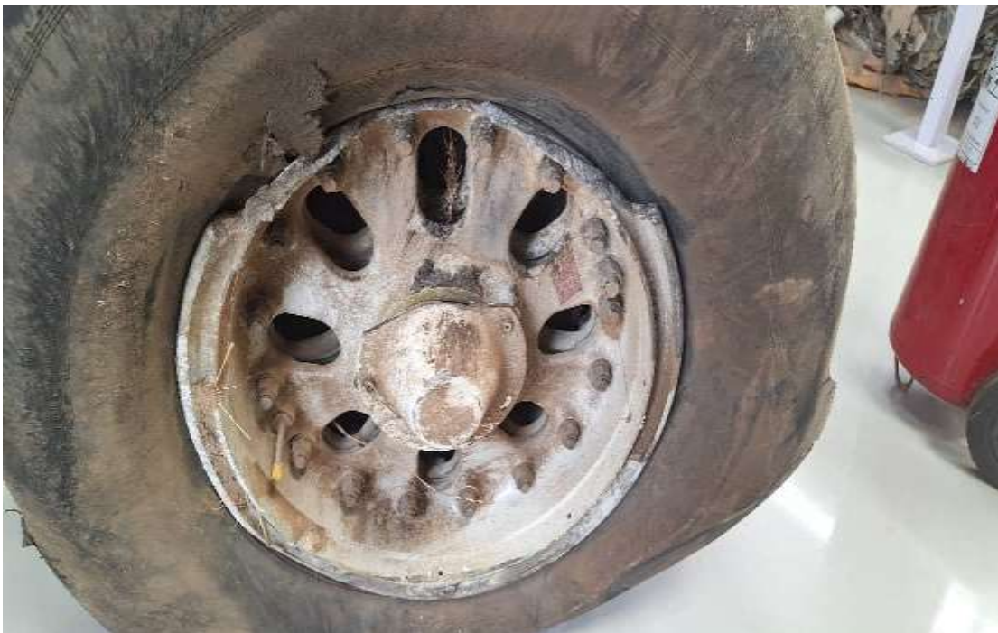
Figure 10: Damaged No.3 Main Wheel Assembly
