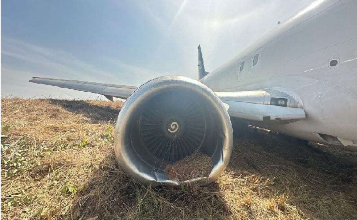
Figure 11: Dents/damage on the No.2 Engine Cowl
