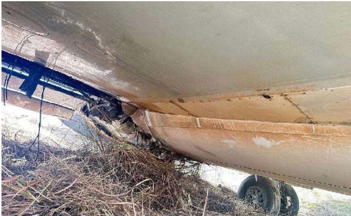
Figure 12: Damage to the lower section of the right-wing
