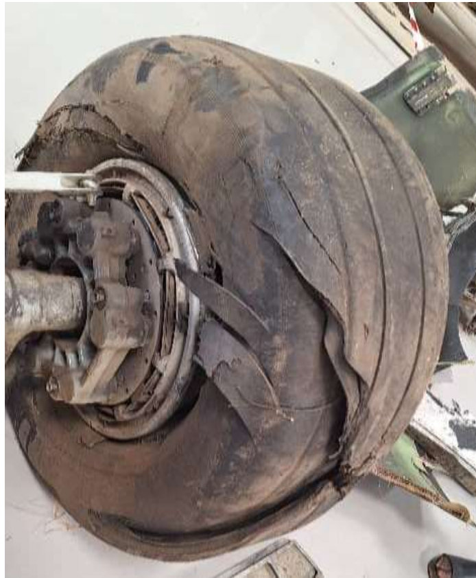
Figure 9: Damaged No.4 Main Wheel Assembly
