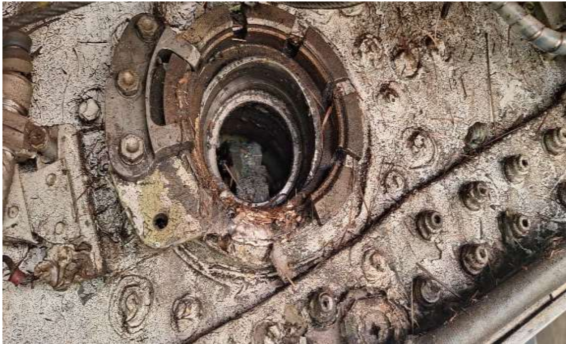
Figure 6: The Joint on the aircraft where the Right Main Landing Gear sheared off
