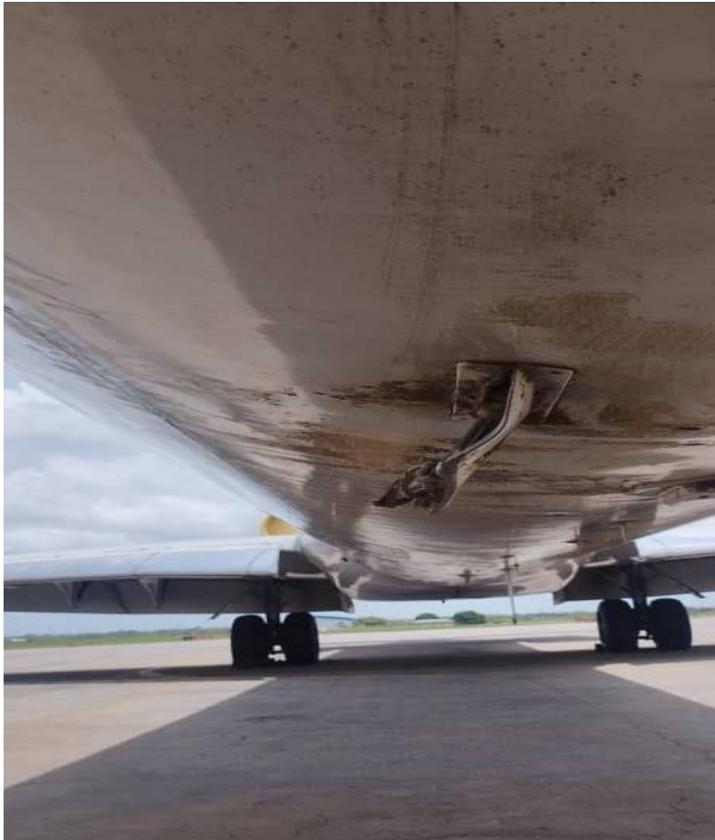
Figure 3: Damaged Galley Drain & Antenna
