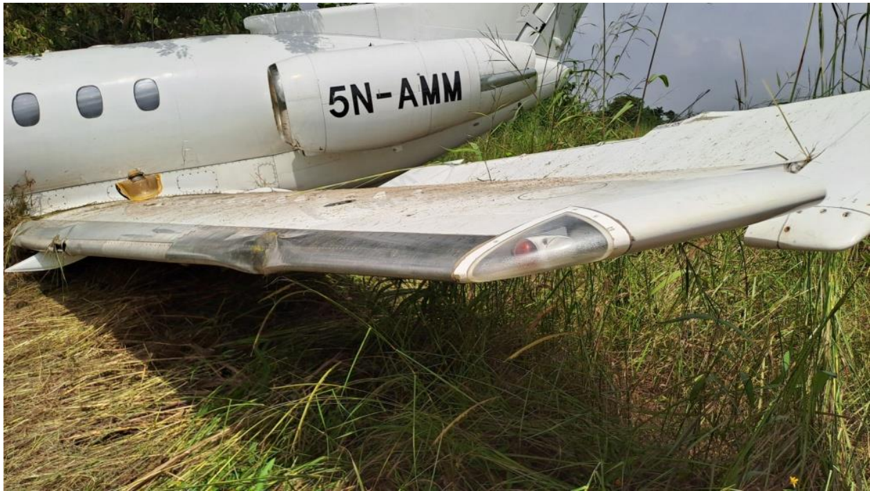
Figure 6: Damage to the left wing leading edge and a fragment of the approach lighting fixture
