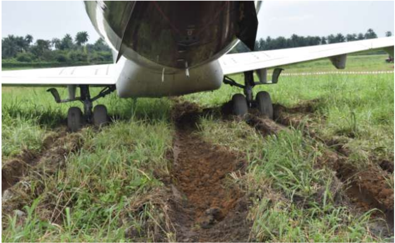
Figure 1: Some views of the aircraft landing gear where it stopped
