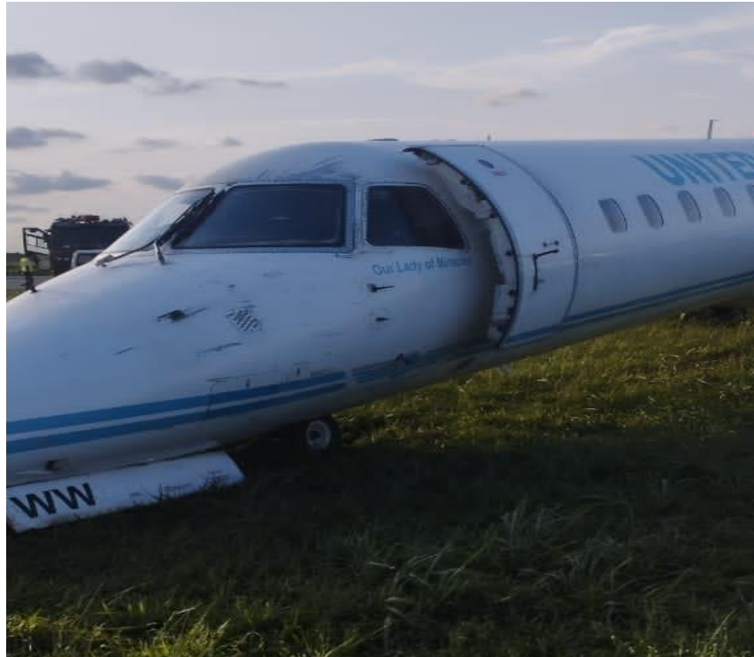
Figure 4: The collapsed nose wheel landing gear
