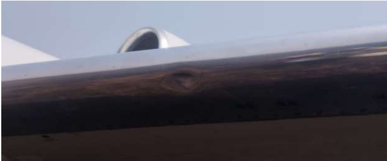
Figure 8: Dent created about the mid-section of left wing leading edge surface
