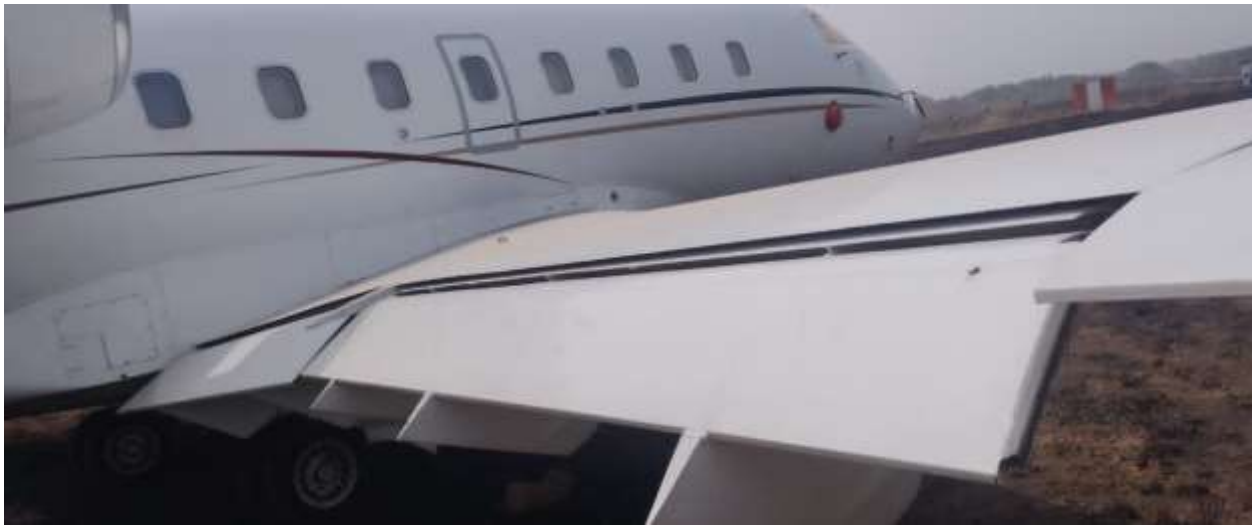
Figure 7: The right-wing flap surface position on landing
