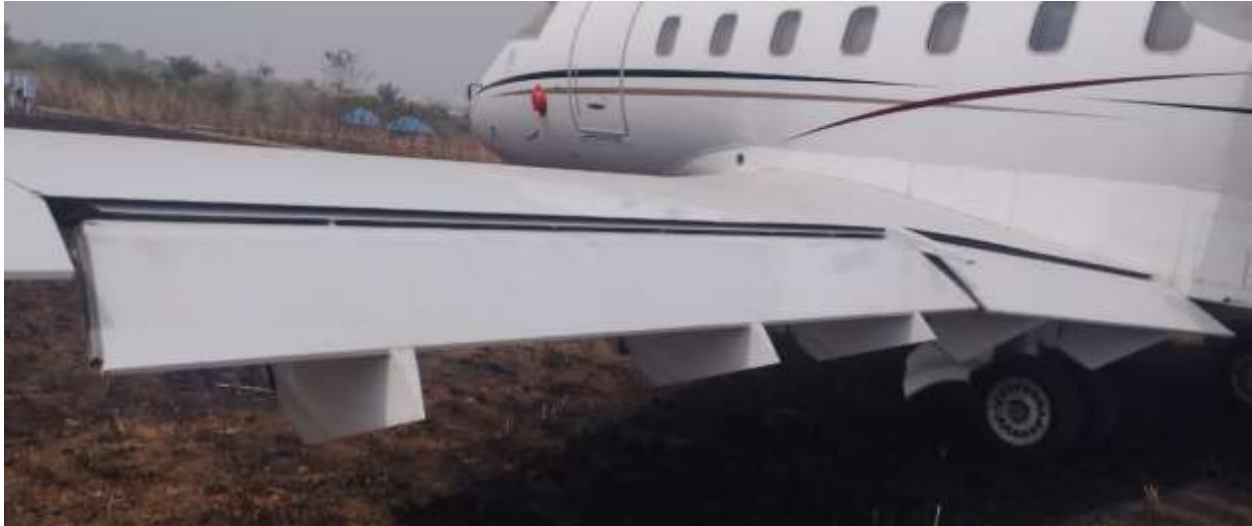
Figure 6: The left-wing Flap surface position on landing
