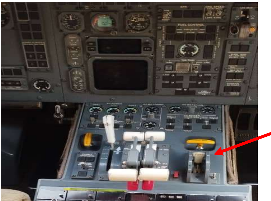
Figure 9: Flap handle Selector position on the flight pedestal
