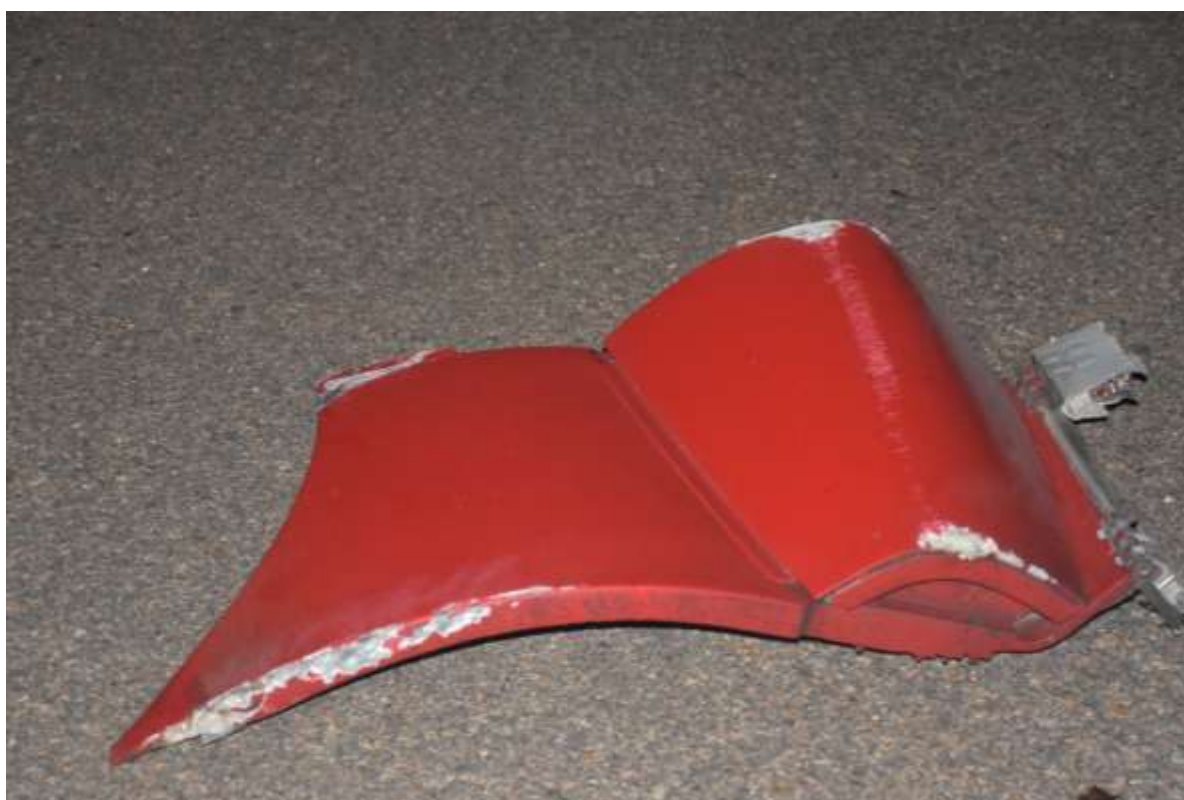
Figure 16: Debris of the damaged nose landing gear
