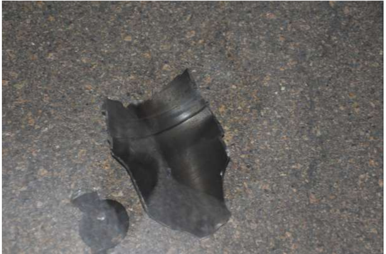
Figure 12: Debris of the damaged nose landing gear
