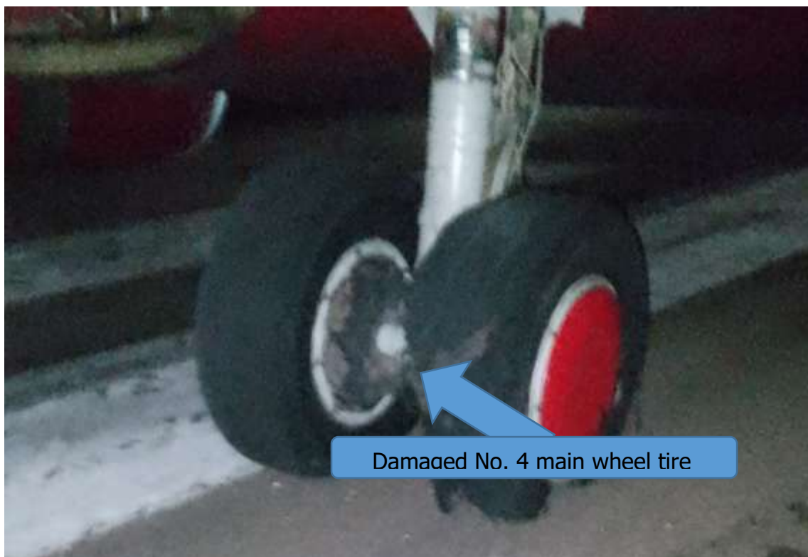
Figure 6: Damaged No. 4 main wheel tire
