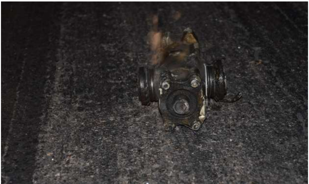
Figure 12: Debris of the damaged nose landing gear
