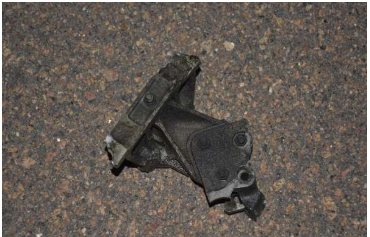
Figure 14: Debris of the damaged nose landing gear
