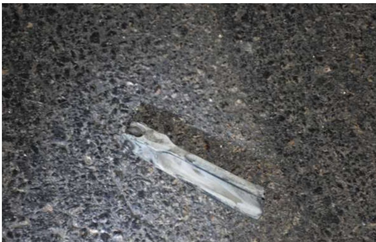
Figure 10: Debris of the damaged nose landing gear
