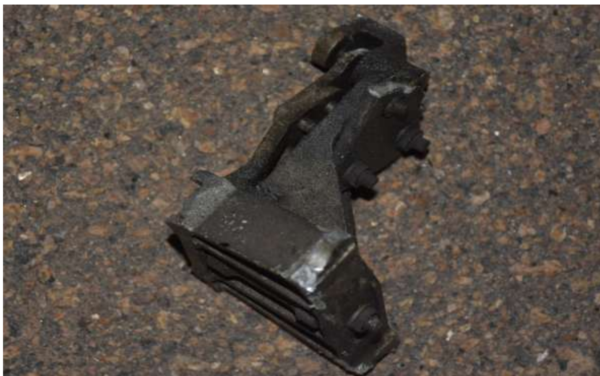
Figure 16: Debris of the damaged nose landing gear
