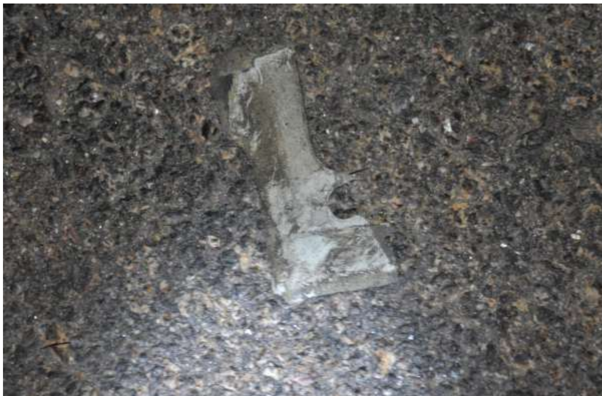
Figure 10: Debris of the damaged nose landing gear
