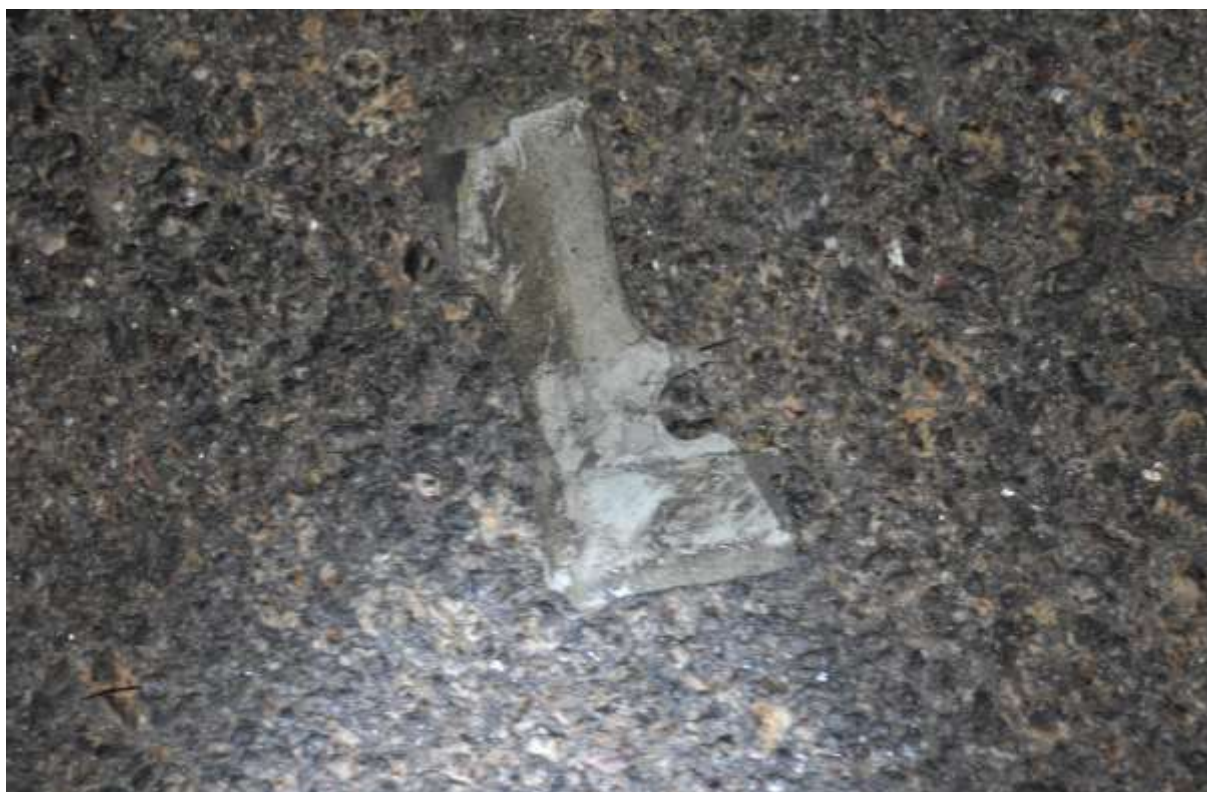
Figure 10: Debris of the damaged nose landing gear
