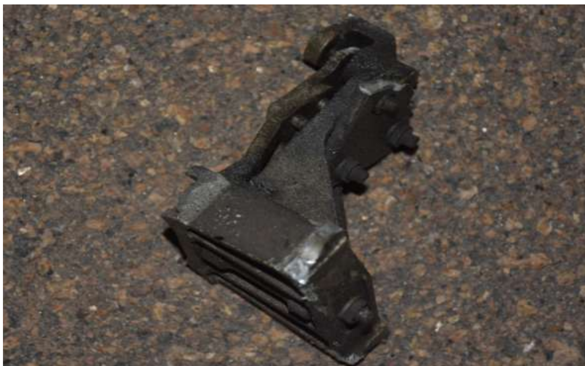
Figure 16: Debris of the damaged nose landing gear
