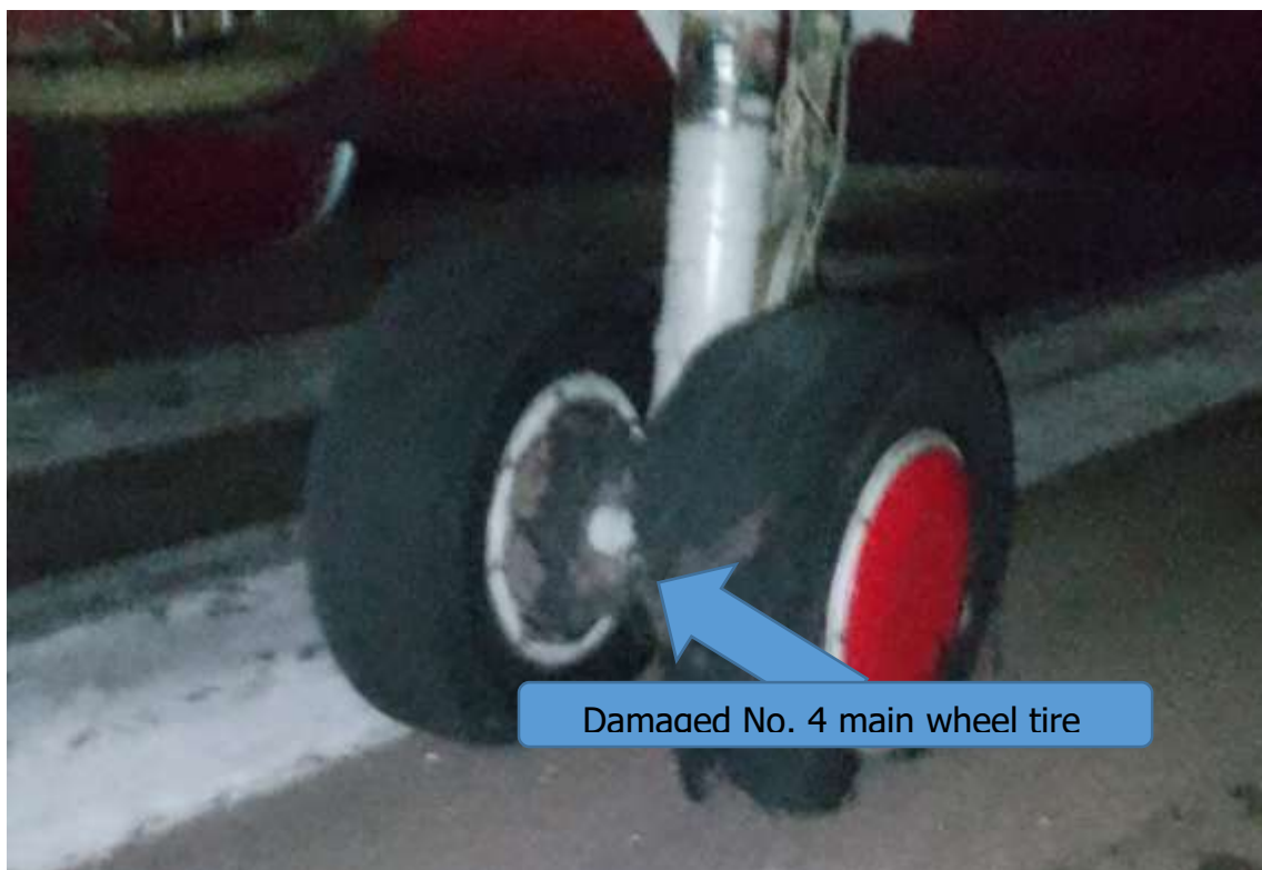
Figure 6: Damaged No. 4 main wheel tire
