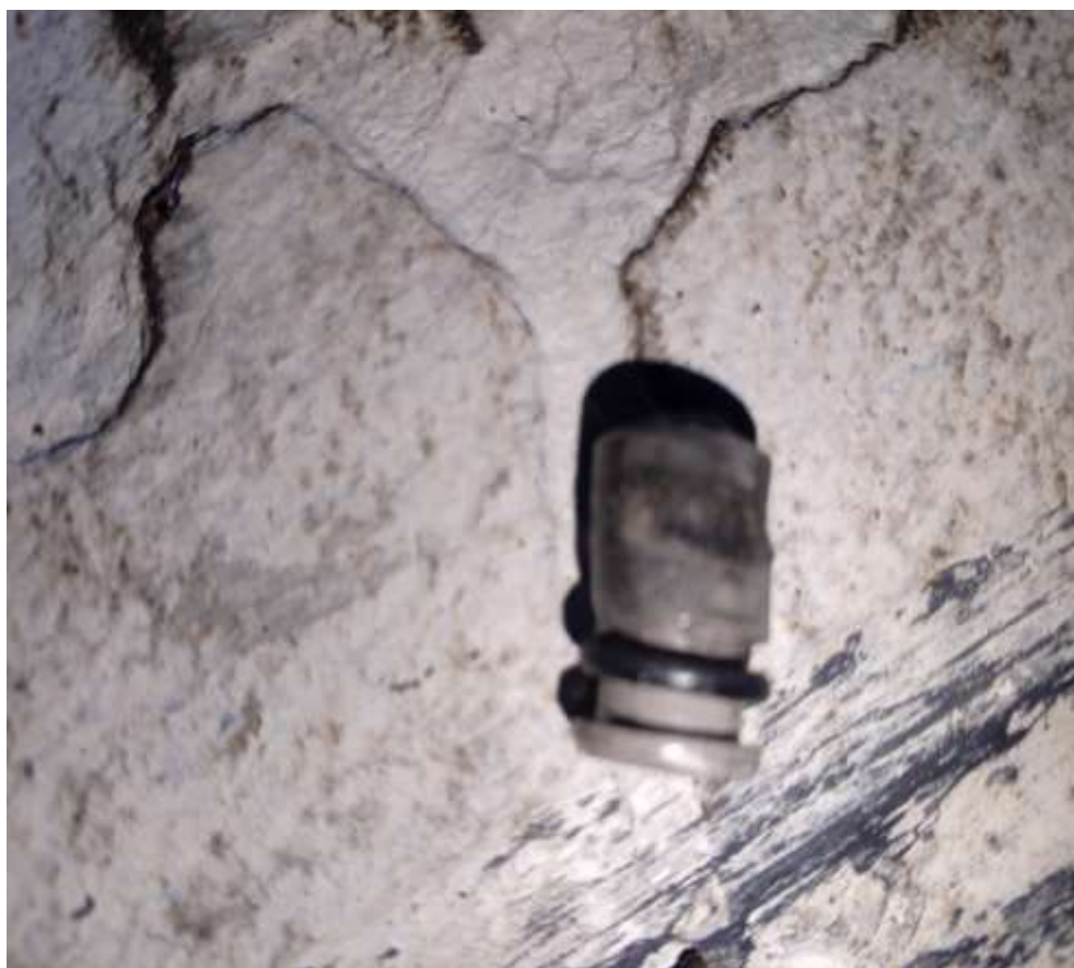
Figure 9: Debris of the damaged nose landing gear
