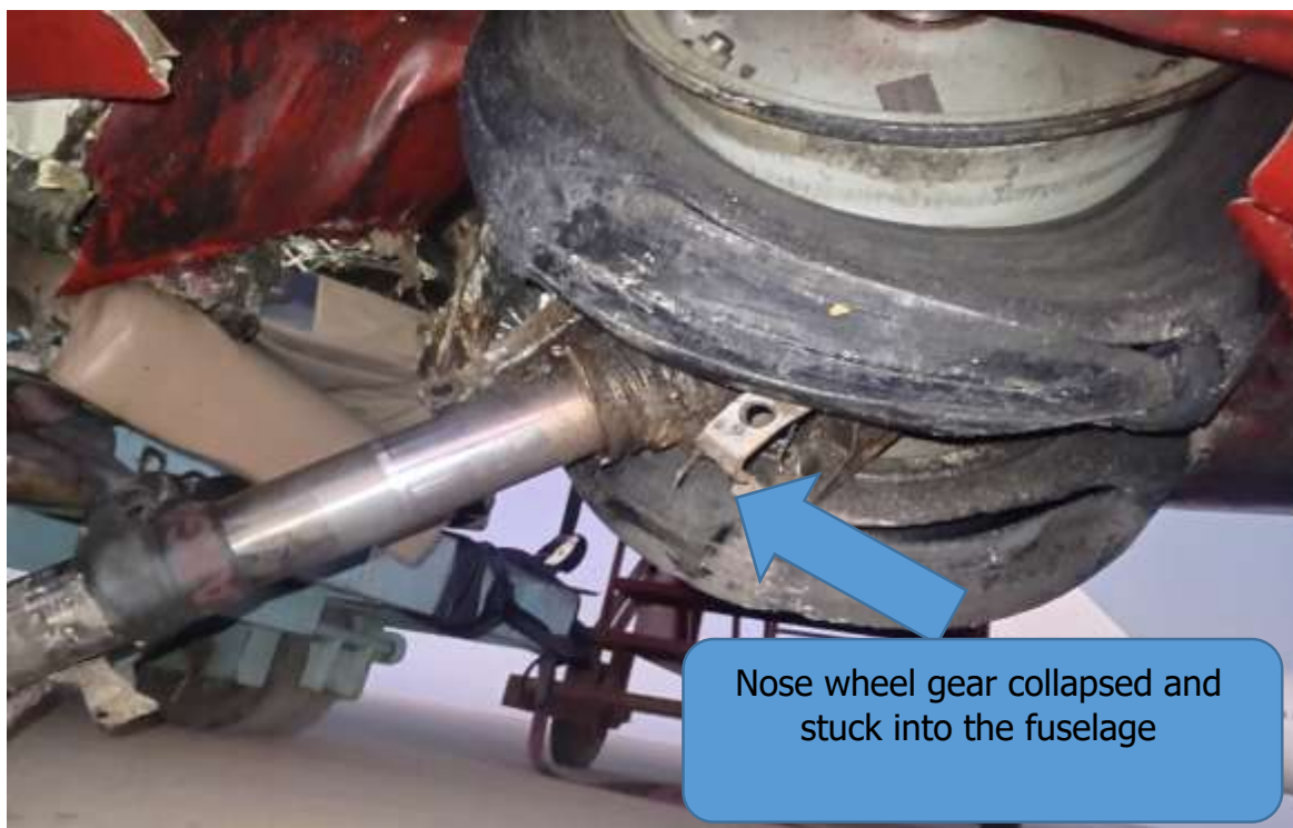
Figure 8: Nose wheel gear collapsed and stuck into the fuselage belly.
