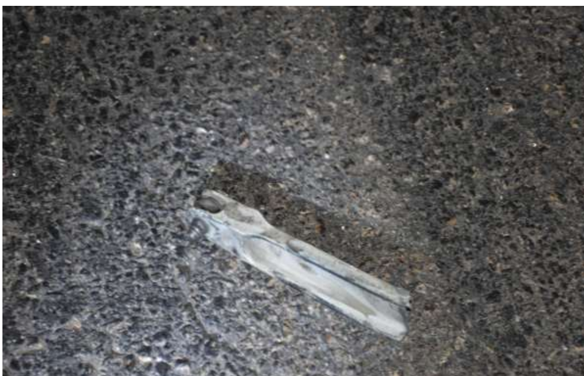
Figure 10: Debris of the damaged nose landing gear
