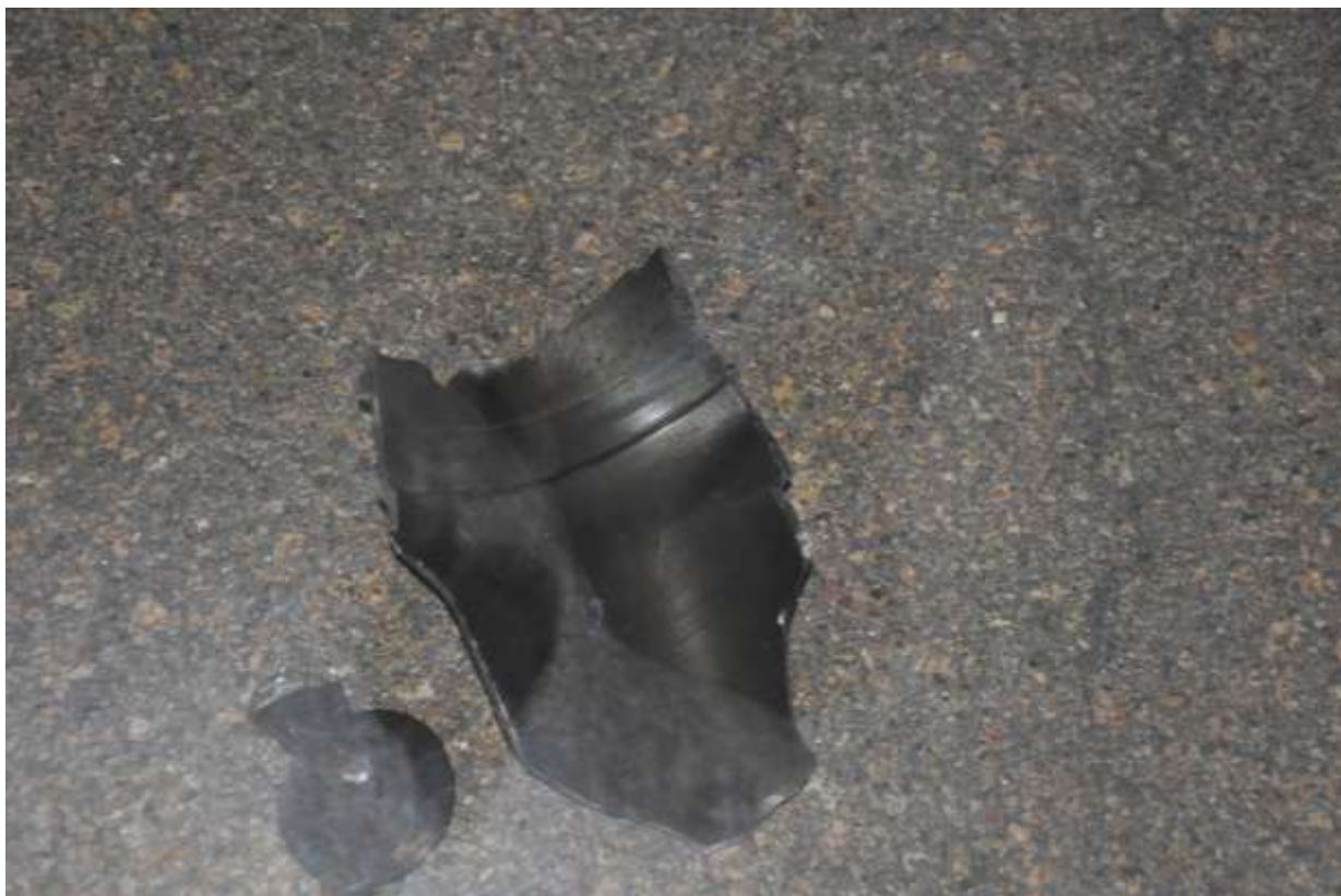
Figure 12: Debris of the damaged nose landing gear
