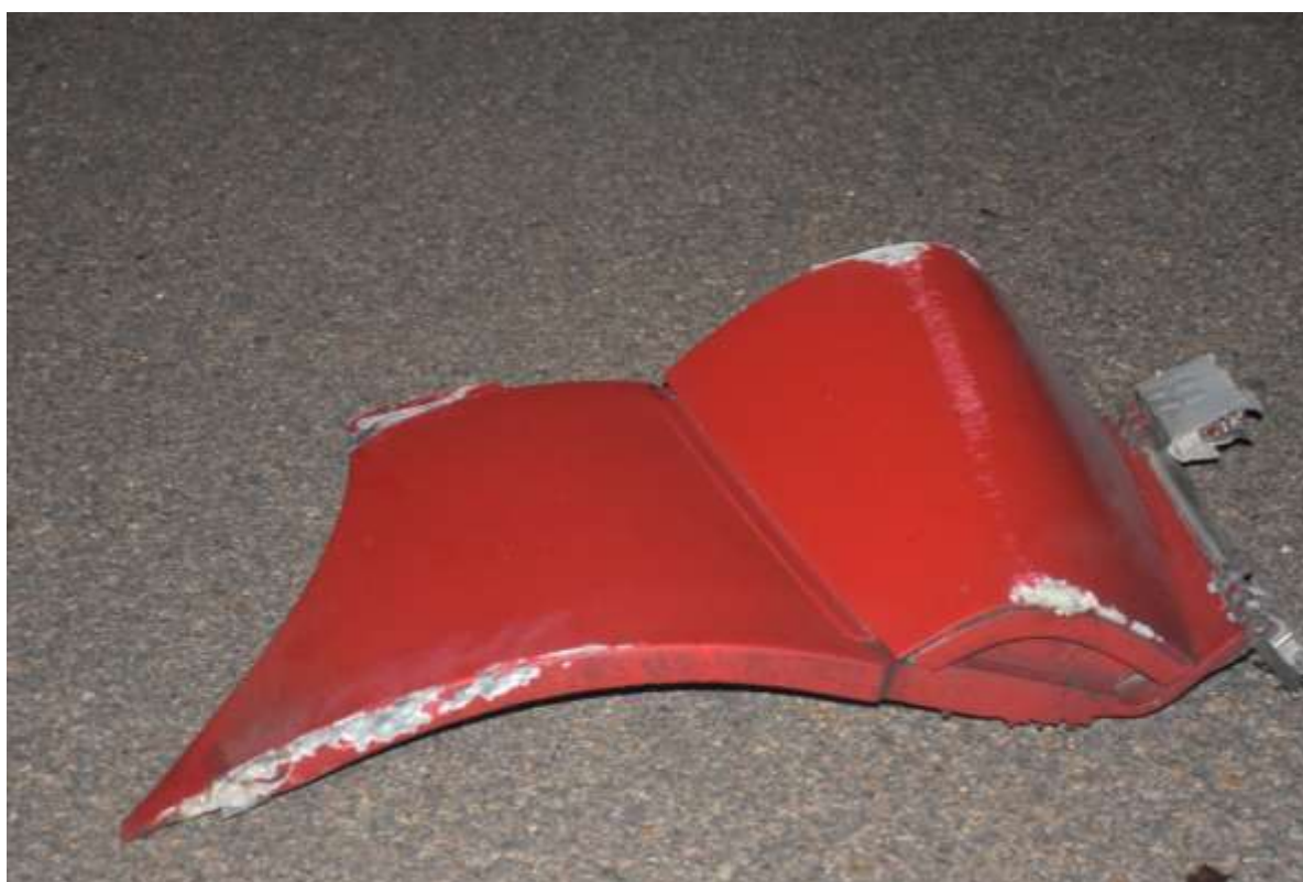
Figure 17: No.2 Main wheel well door
