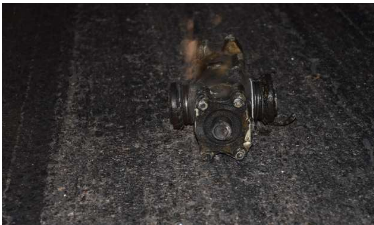
Figure 12: Debris of the damaged nose landing gear
