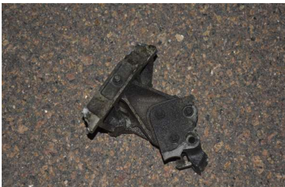
Figure 14: Debris of the damaged nose landing gear
