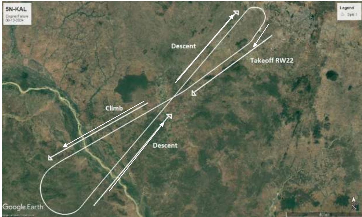
Figure 1: Flight track for 5N-KAL as obtained from position data from the Flight Data Recorder
