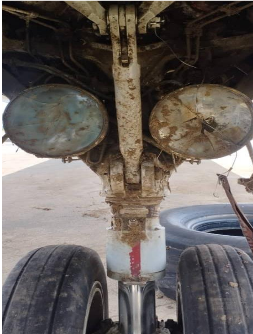
Figure 4: Damaged nose landing gear light
