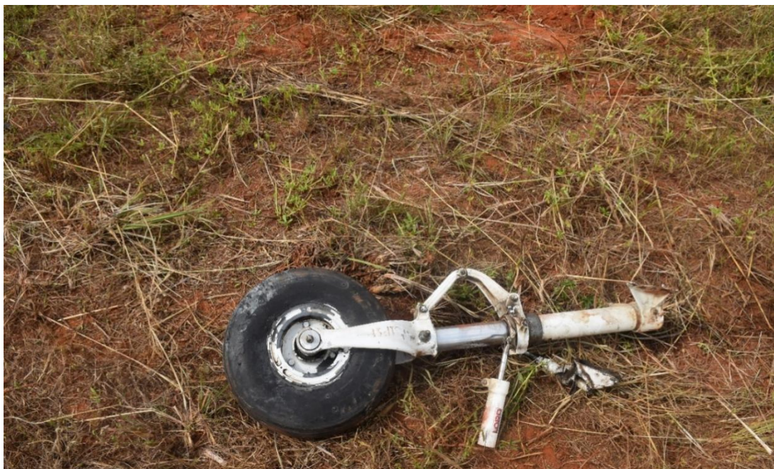
Figure 8: The detached nose landing gear
