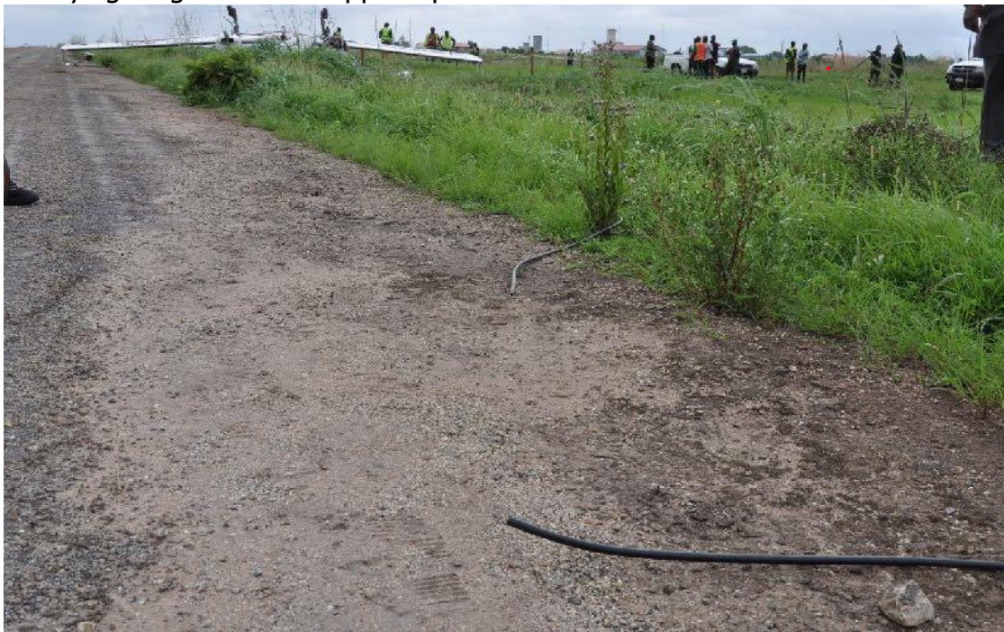
Figure 1: Ripped runway lighting cable
