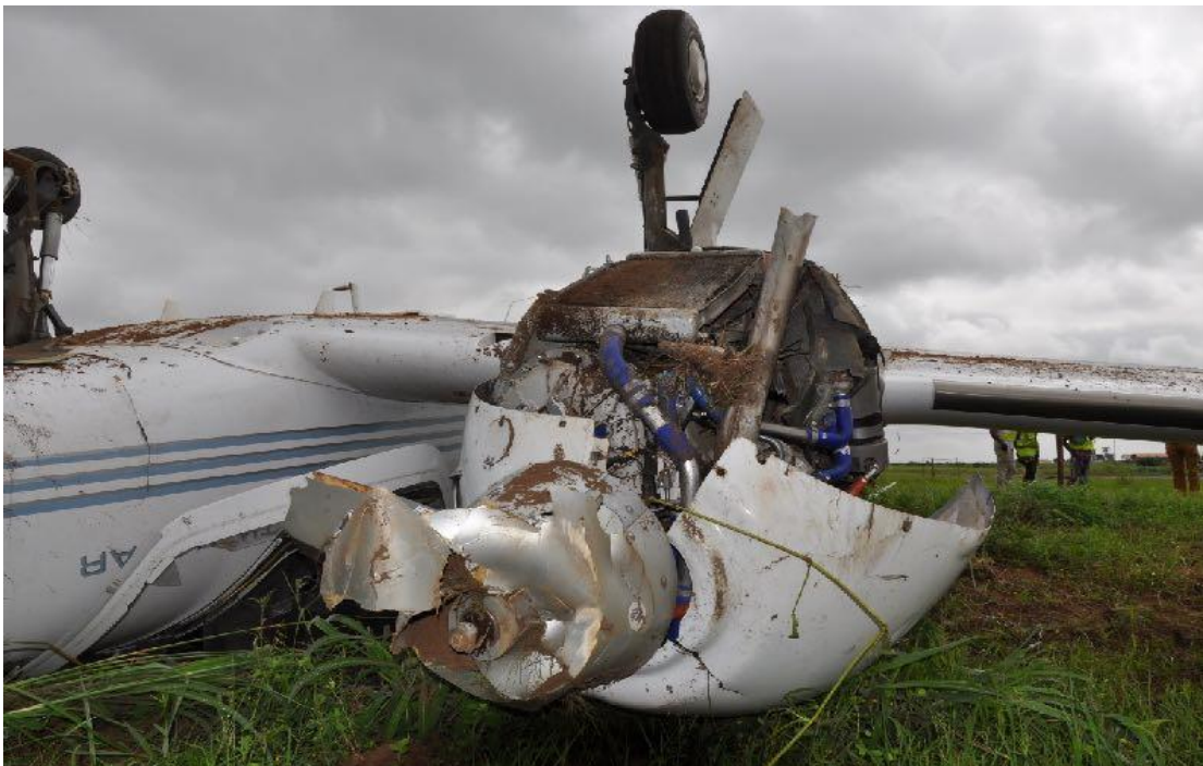
Figure 7: Broken propeller blades on LH engine
