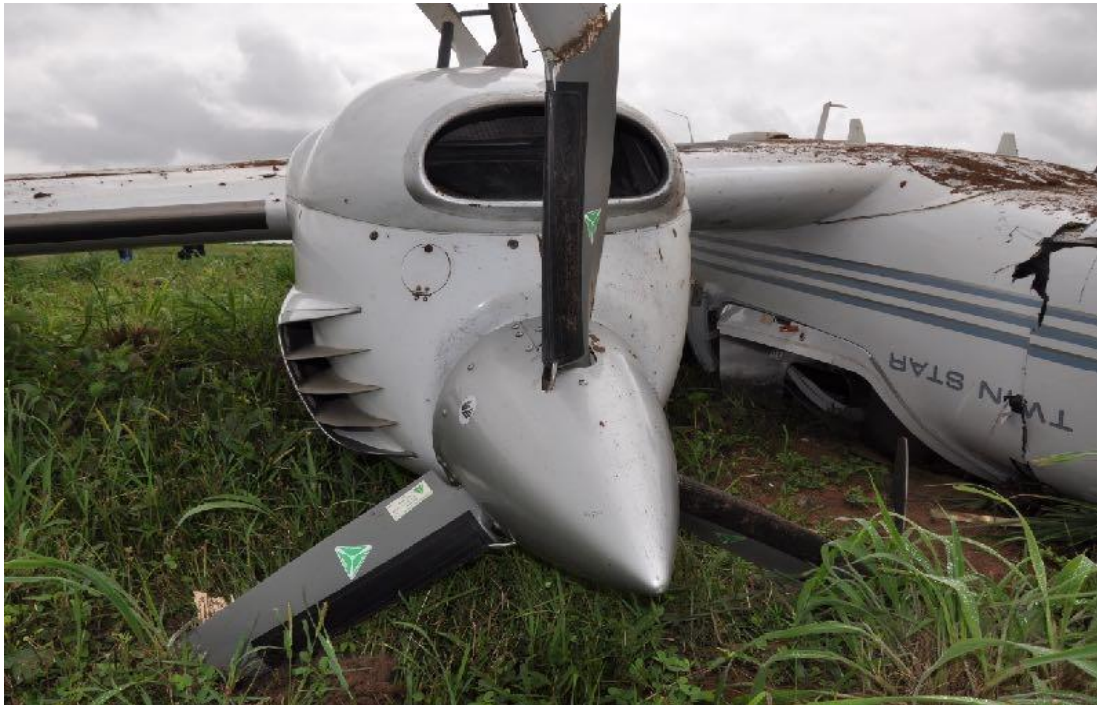
Figure 7: Broken propeller blades on LH engine
