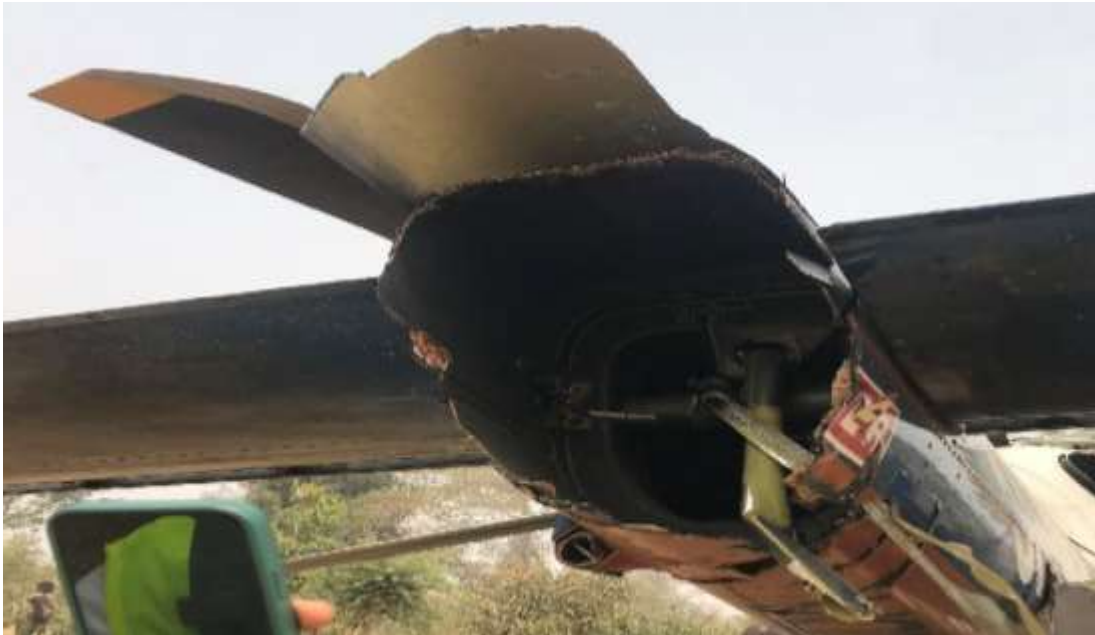
Figure 4: Broken Tail Boom
