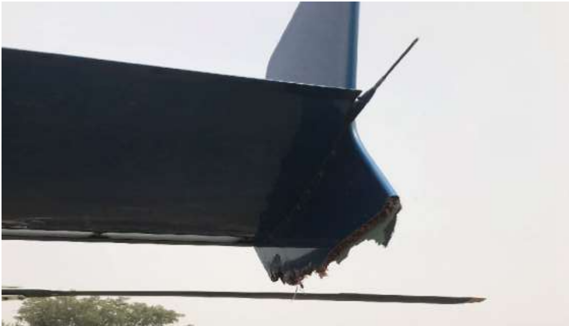
Figure 6: Damaged Vertical Stabiliser
