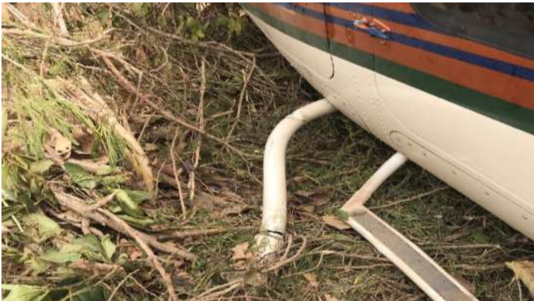
Figure 5: Collapsed left side Skid
