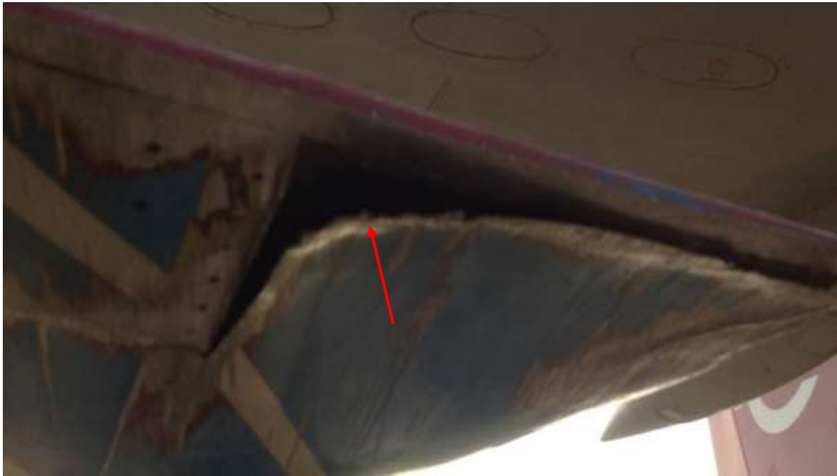
Figure 16: The ruptured right tank from the bottom
