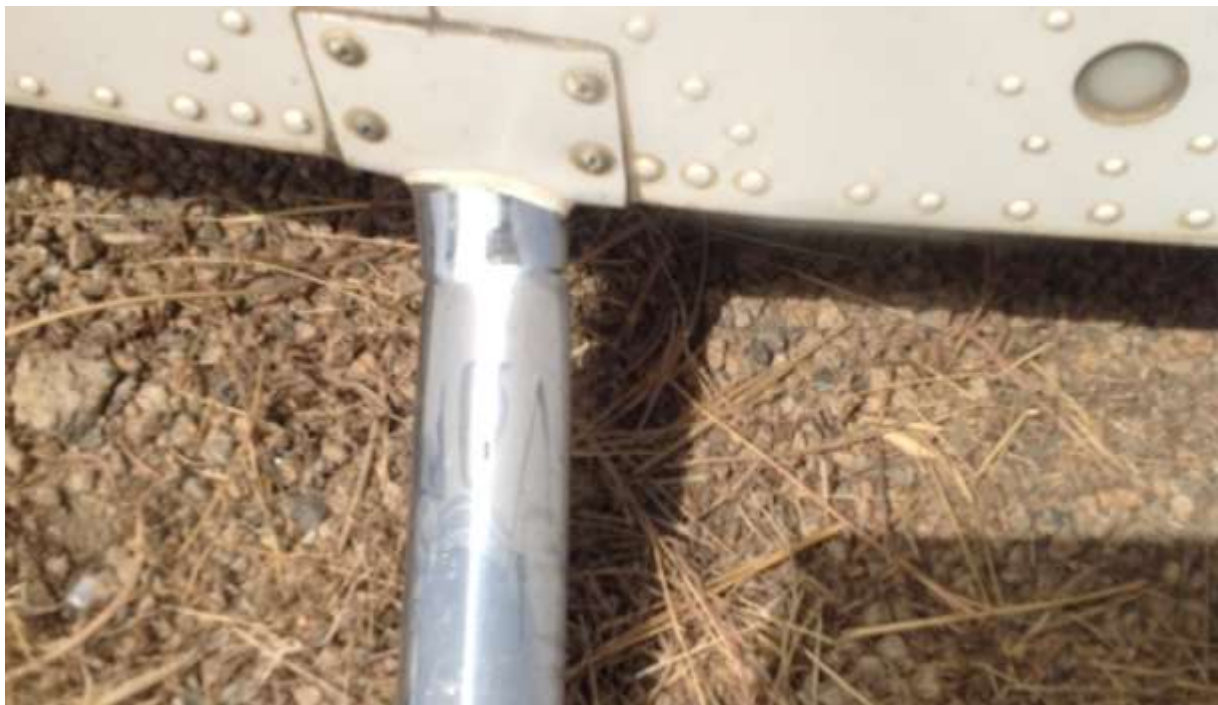
Figure 15: The broken right door step
