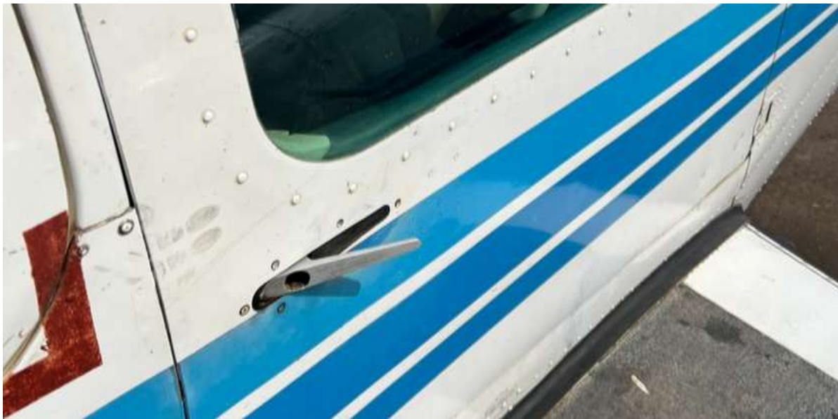
Figure 2: The unlatched starboard door handle
