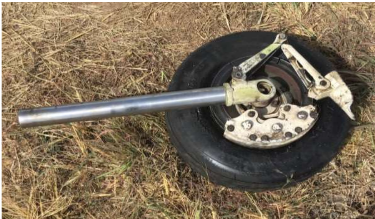
Figure 11: The sheared right main landing gear
