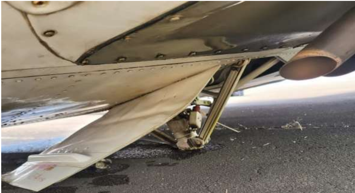
Figure 12: The remaining part of the landing gear attach to the aircraft
