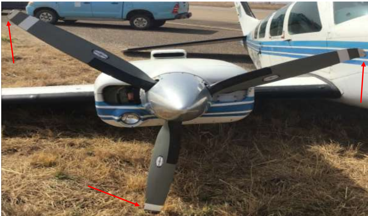
Figure 14: Bent propeller blade at the tip
