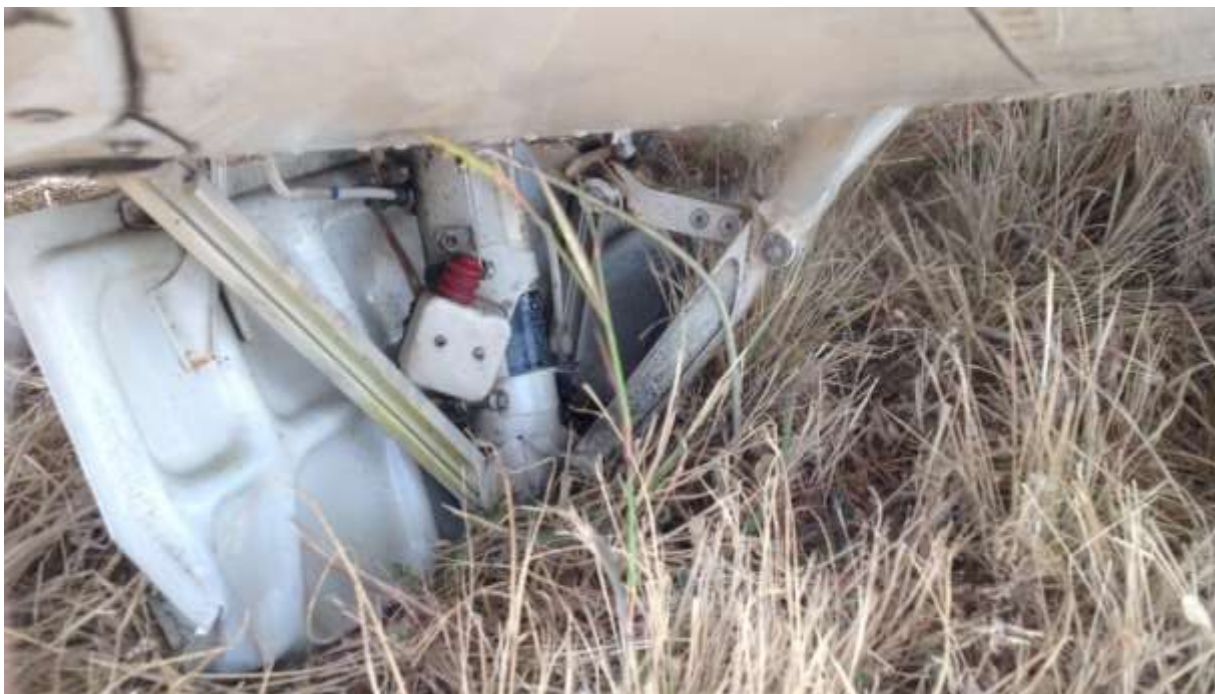
Figure 13: The remaining part of the landing gear attach to the aircraft after it was moved
