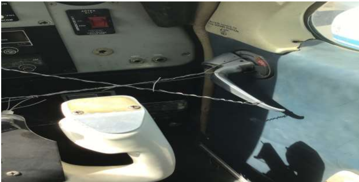
Figure 3: The starboard door locked from inside the cockpit
