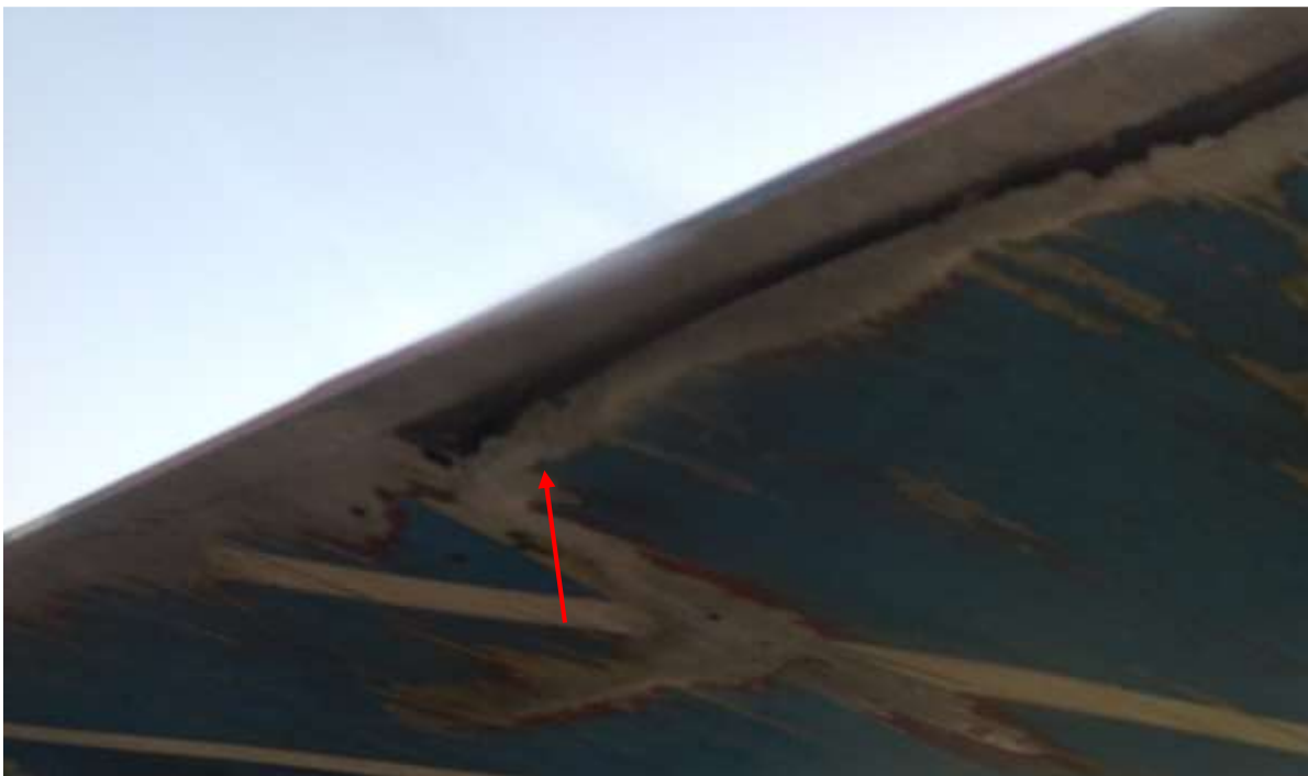
Figure 17: The ruptured right tank from the bottom
