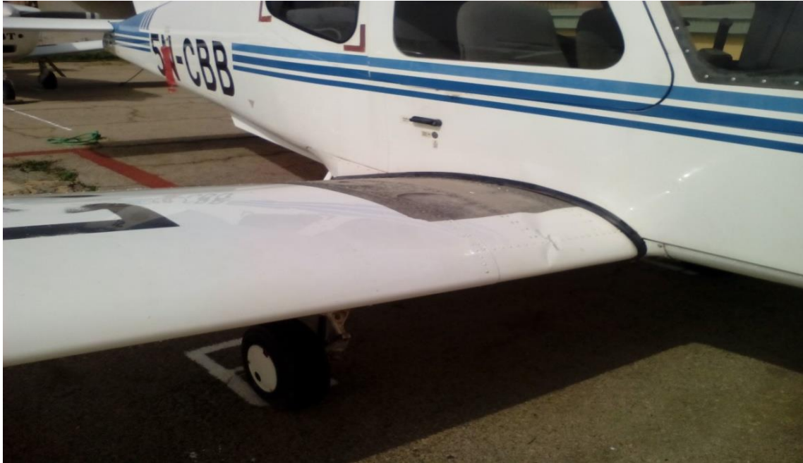
Figure 1: Dent on the right wing skin at the root end.
