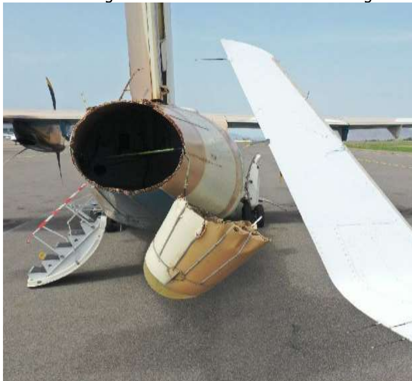
Figure 10: Damaged Section of the Tail Cone of ATR (NAF930)
