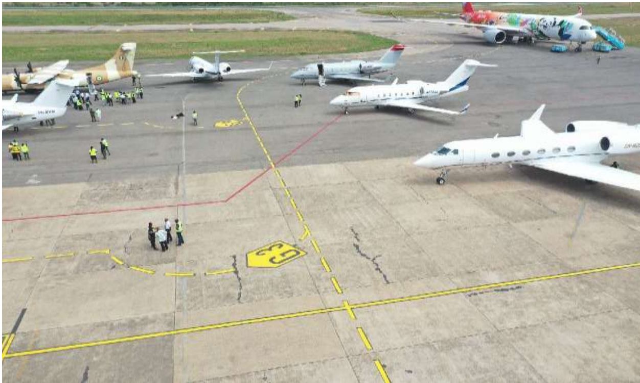
Figure 7: NAF ATR 42 parked at unmarked spot with its Tail Section protruding into the Apron Taxi Lane used by 5N-BXK. Other aircraft parked at unmarked spots on the GAT/Cargo Apron right side of 5N-BXK
