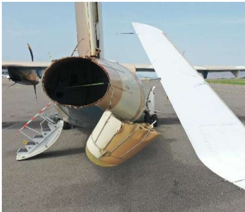
Figure 2: Sheared off section of the Tail cone of the parked ATR 42 (NAF930)
