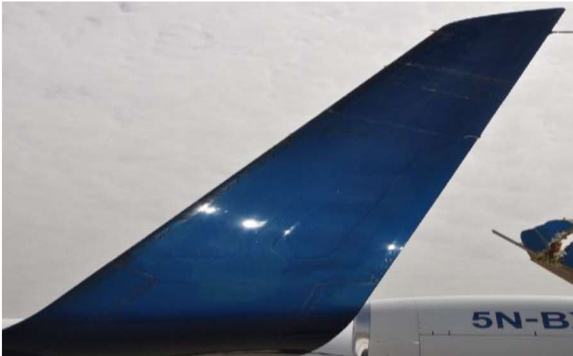
Figure 9: 5N-BXK Winglet abrasion and the broken discharge wick position
