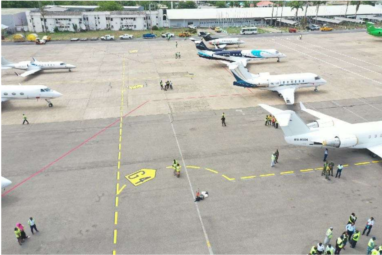
Figure 5: Aerial view of congested GAT/Cargo Apron with aircraft parked at marked positions and at unmarked spots on both sides of the Apron Taxi Lane used by 5N-BXK.
