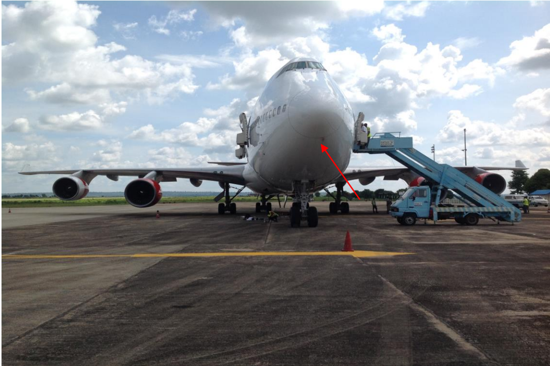
Figure 7: Bird strike at the edge of the radome
