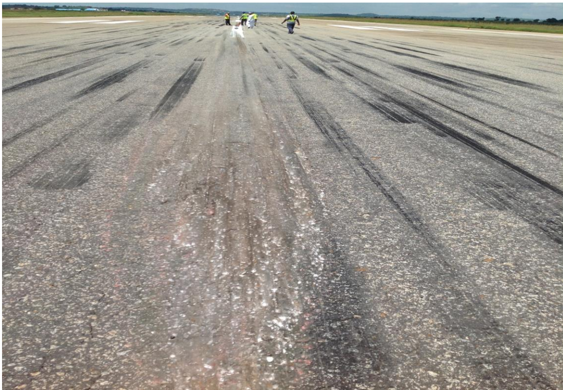
Figure 4: Impact marks of engine number 1 on runway centerline
