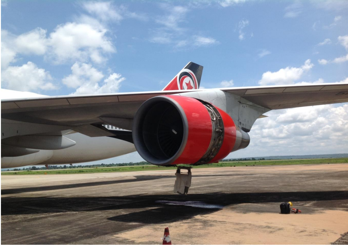
Figure 2: Damage to the left cowling of engine number one
