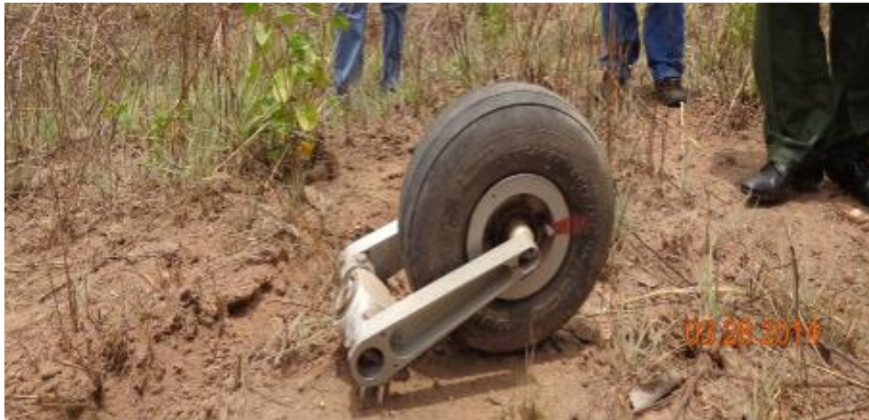
Figure 3: Photo of the broken nose wheel
