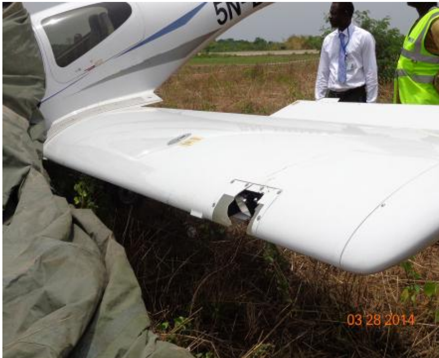
Figure 1: Photo of damaged landing light on port wing
