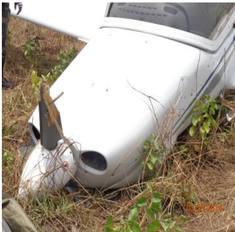
Figure 6: Photo of the aircraft's forward fuselage and broken propeller blades
