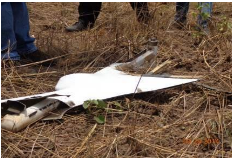
Figure 2: Photo of sheared-off Nose Landing Gear
