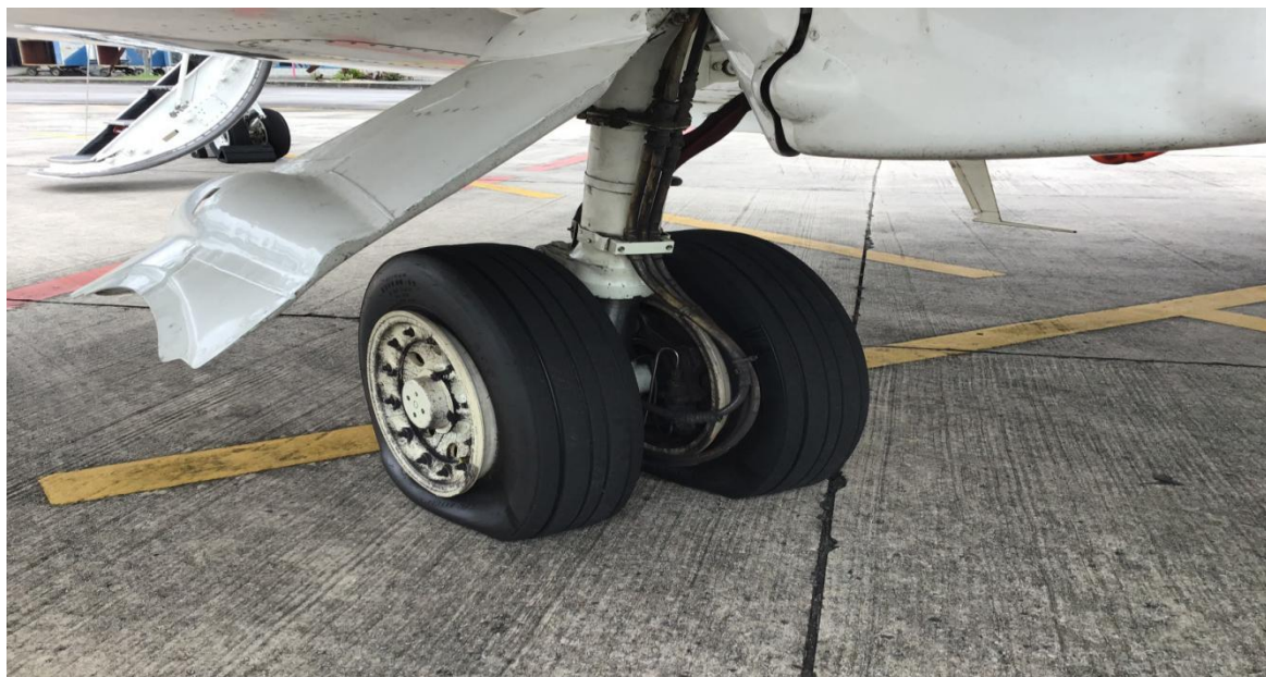
Figure 1: The left main wheel tyres (No.1 and No.2) deflated
