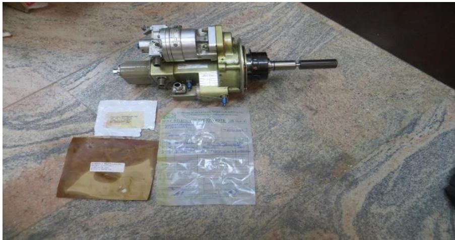
Figure 6: The defective left engine PCU
