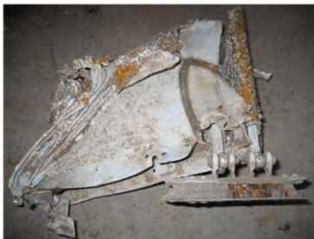
FIG 46A Bottom View RH aileron partial - containing tab push rods and tab mast fitting.
