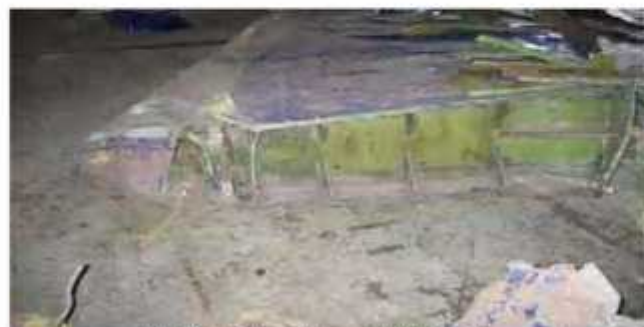
FIG 27A Inboard view of R/H Stabilizer
