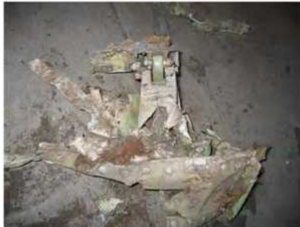
FIG 45A Plan View of the hinge shown in Fig. 2. Fixed trailing edge aileron hinge fitting. (ref D6-15897 pg 54).
