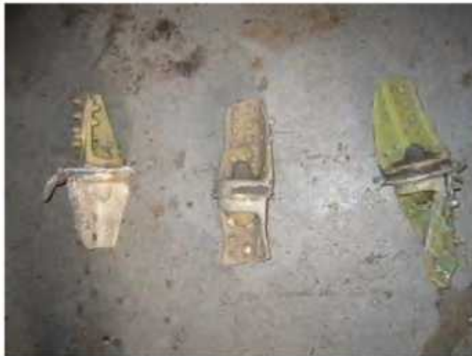
FIG 57 - 65-45437 series tension beam brackets on wing center section spanwise beam instal
