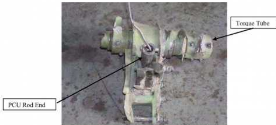
FIG 18 – Elevator Input Torque Tube & PCU Rod End
