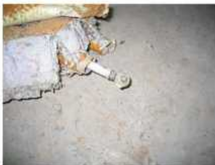
FIG 46B Aux View RH aileron (partial) - containing tab push rods at forward end.
