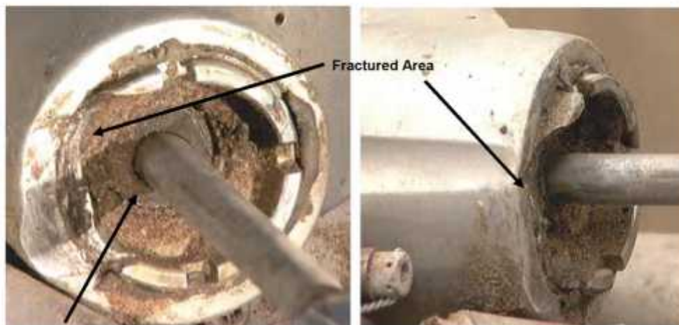
"Recessed" aft piston rod Figure 15
