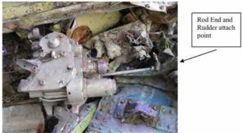
FIG 14 – Main Rudder PCU (at impact site)
