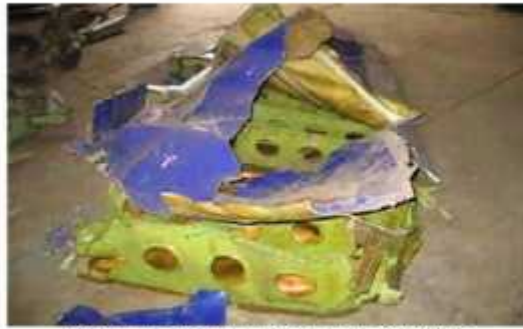
FIG 34 Inboard View of Damaged Stabilizer
