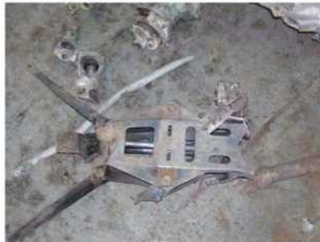
FIG 25 – One of four recovered TR actuation mechanisms
