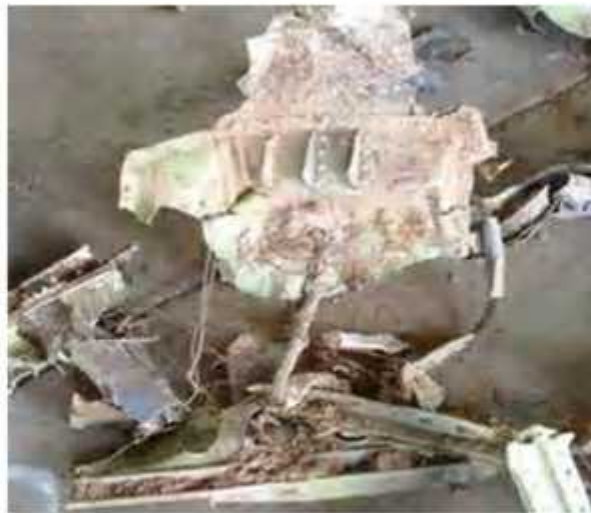
FIG 4 - Aft Pressure Bulkhead Lowest Portion
