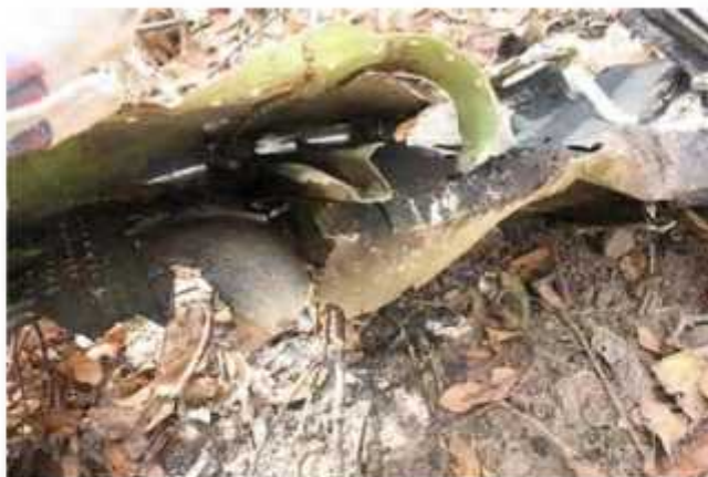
FIG 13B – Burned Part Looking at Inside Fold. Note fire/soot damage stopping within the fold
