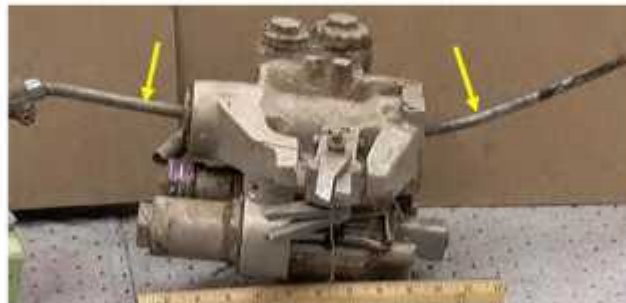
Figure 3. Left side view showing bent, redundant piston rod
