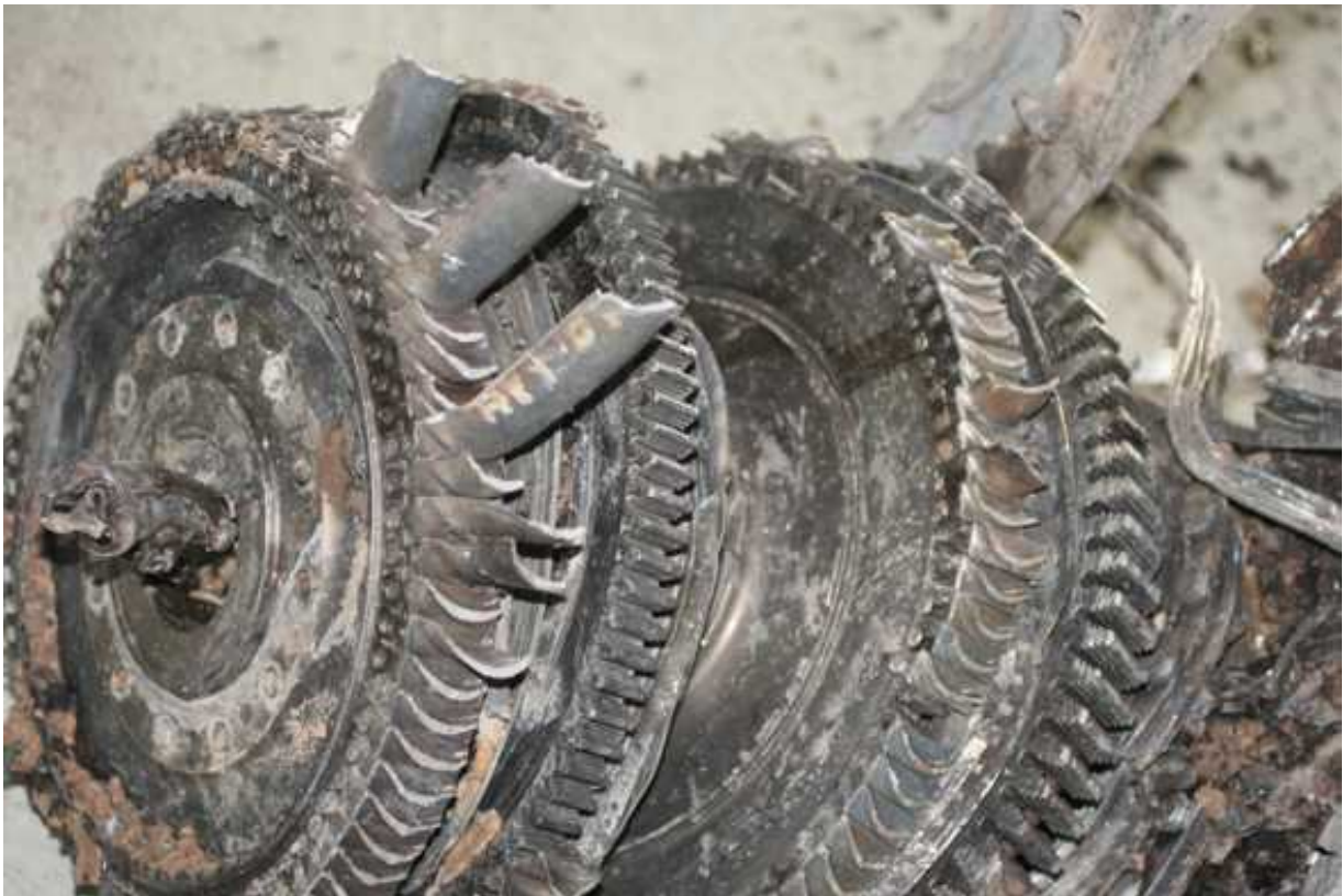
Fig 1.12b An impact damaged engine
