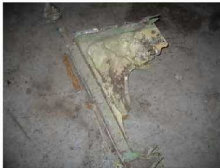
FIG 47B Plan View LH wing tip lower skin with rear spar lower chord horizontal flange shown on the left.
