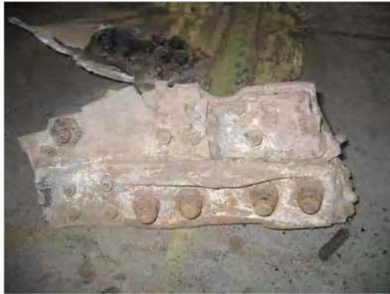
FIG 49B LBL 70.85 lower rear spar chord splice looking down and forward
