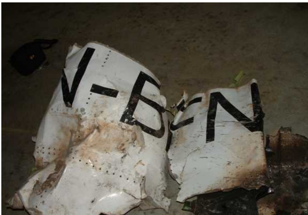
Fig.1.6.1 Two piece match from the left side of the fuselage.
