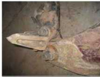
FIG 60A LH main landing gear support beam inbd end – split on bond line. Shown attached to the swing link and body frame.
