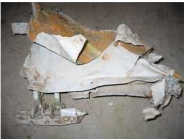
FIG 46 Plan View RH aileron partial - containing tab push rods and tab mast fitting.
