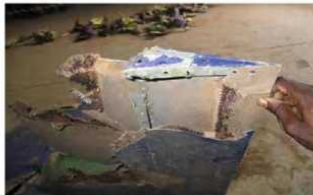
FIG 31A Edge of elevator at the tab cutout
