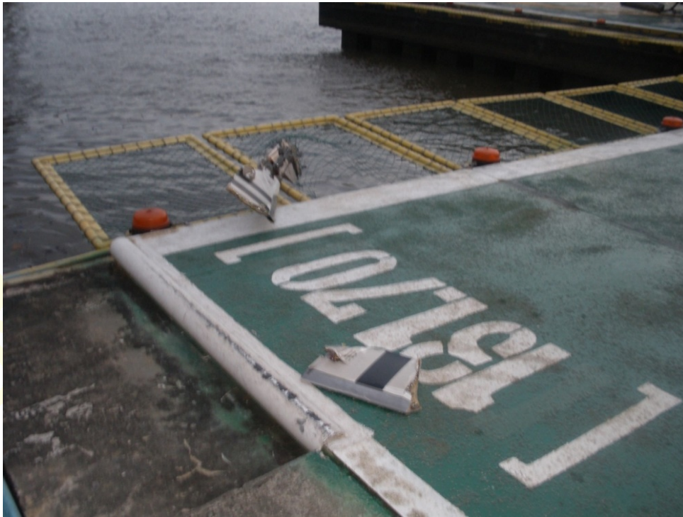
Figure 10: The detached and broken Tail Rotor blade assembly of 5N-BGS on the Helipad
