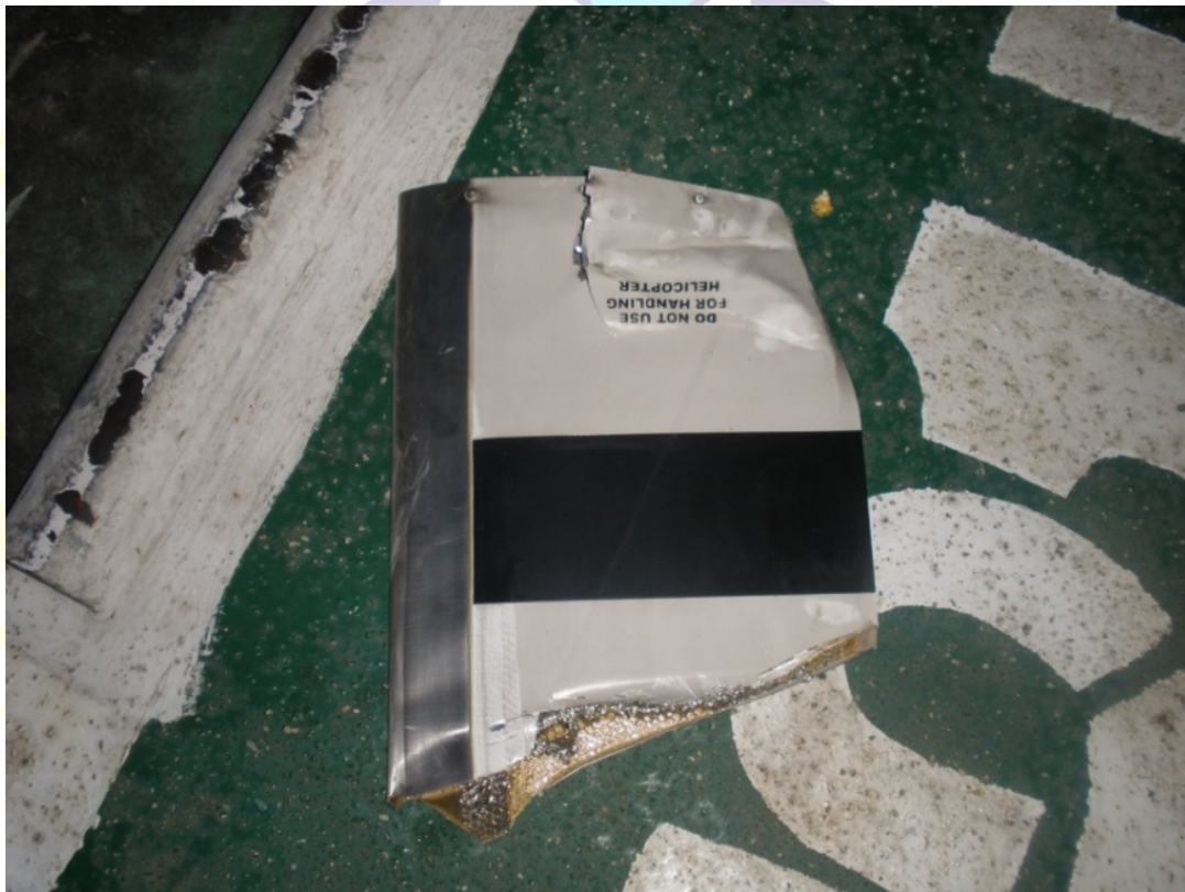
Figure 8: The stump of sheared Tail Rotor blade of 5N-BGS on the Helipad
