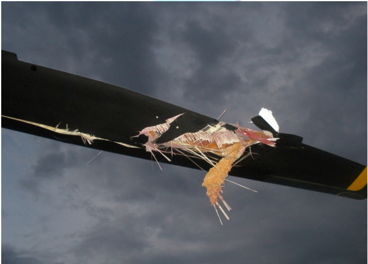
Figure 5: The close-up view of the damage on 5N-BDD Main Rotor
