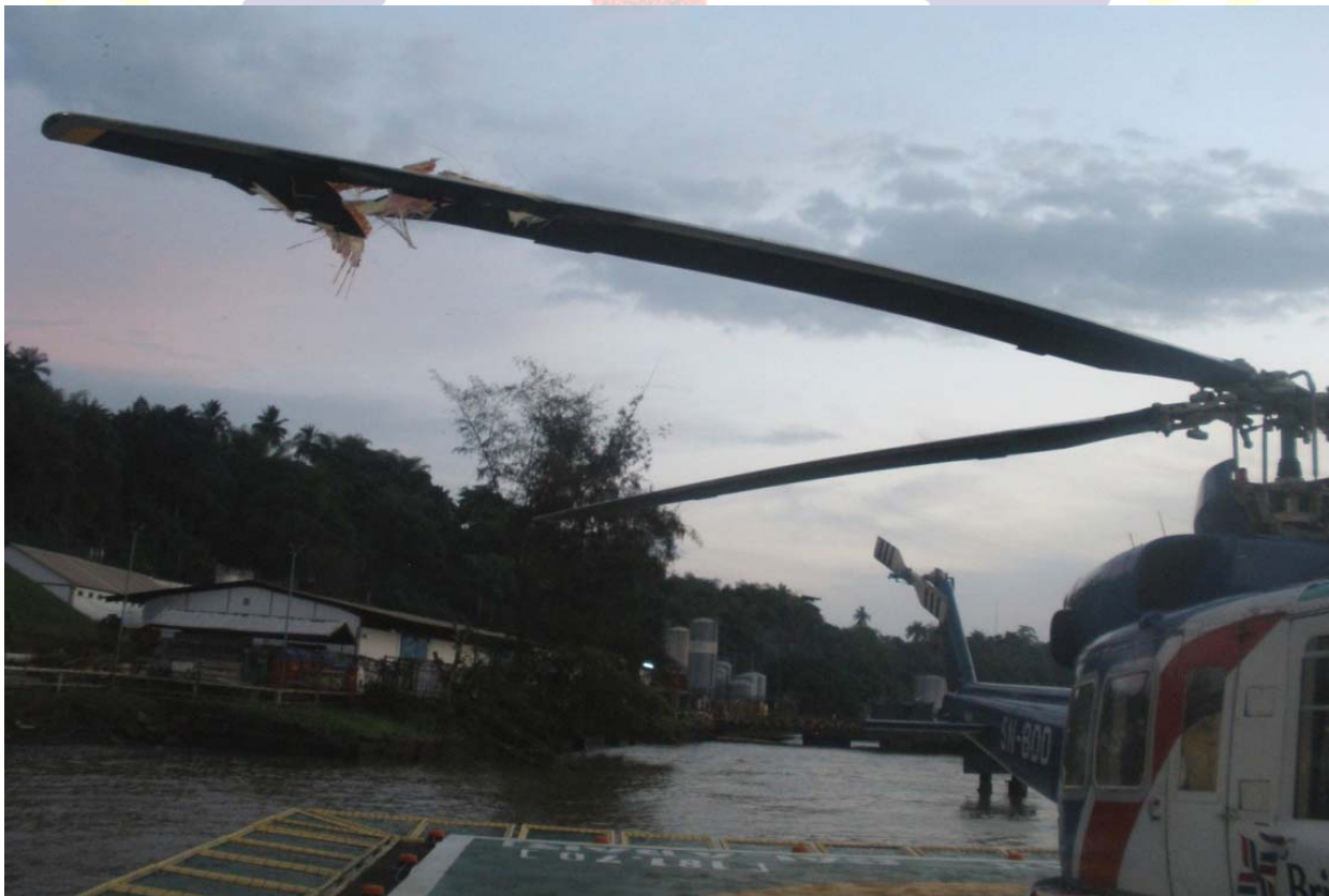
Figure 4: The damaged Main Rotor Blade of 5N-BDD
