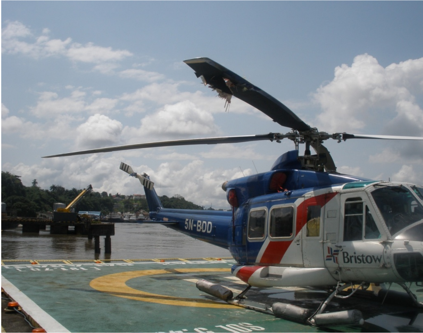
Figure 11: The damage on one of the Main Rotor blade of 5N-BDD on the parking circle
