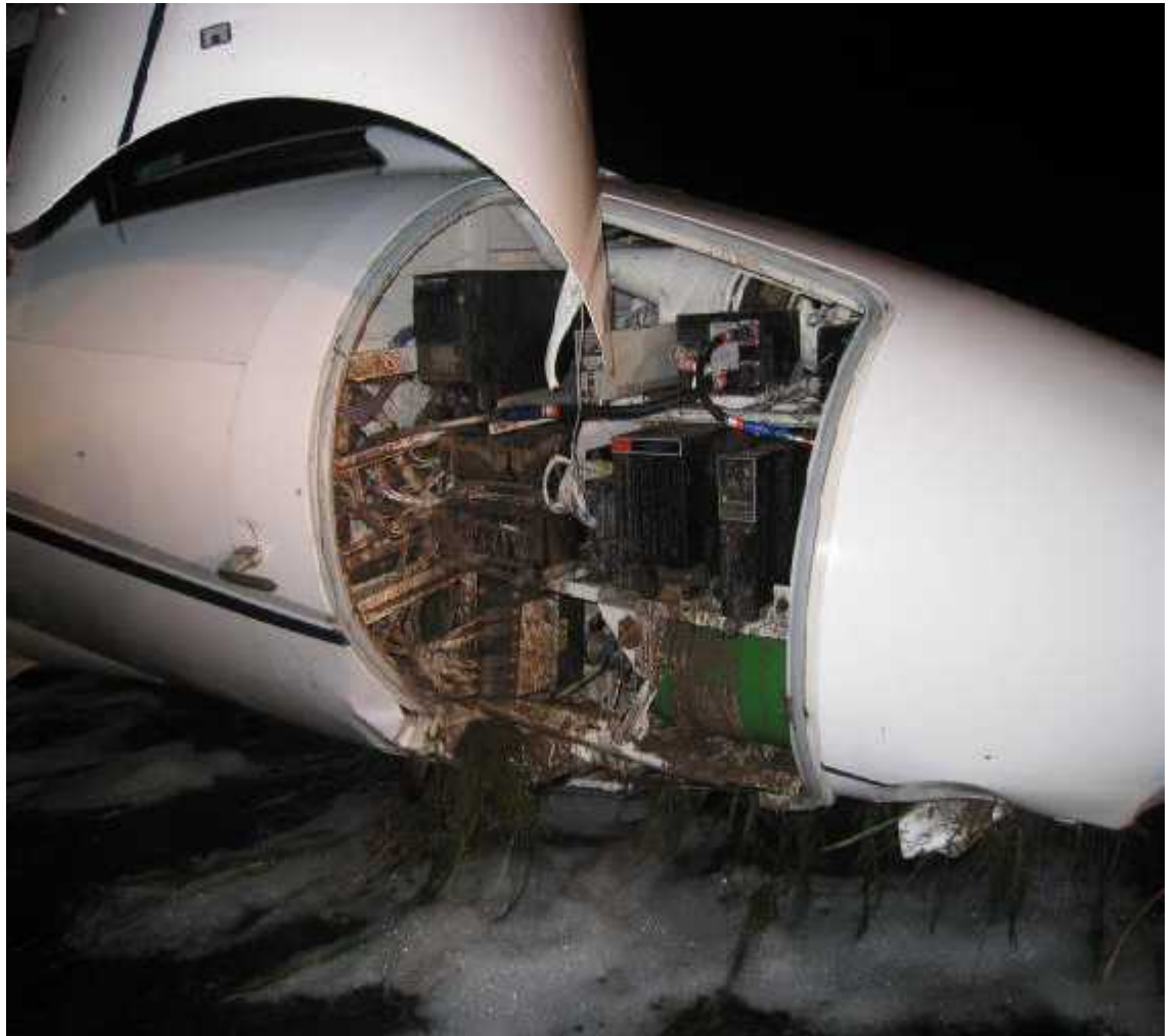
Fig 1.3b Damaged E and E Compartment
