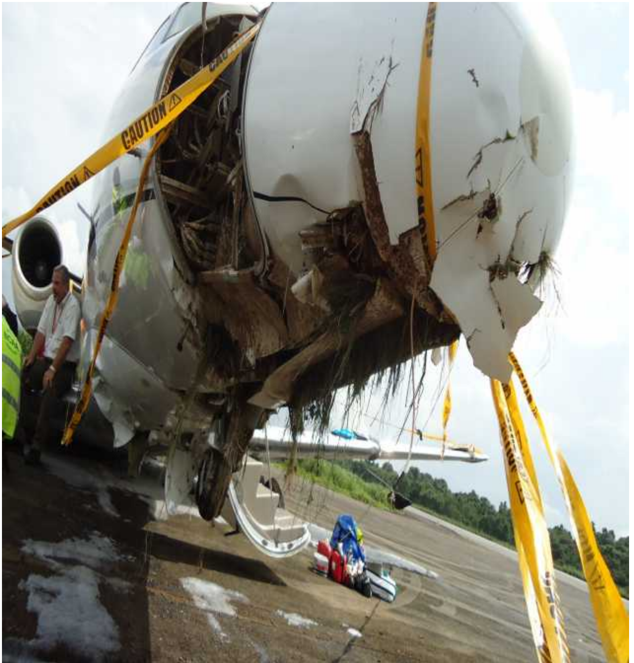
Fig. 1.12b The wreckage showing damaged Radome and Nose section
