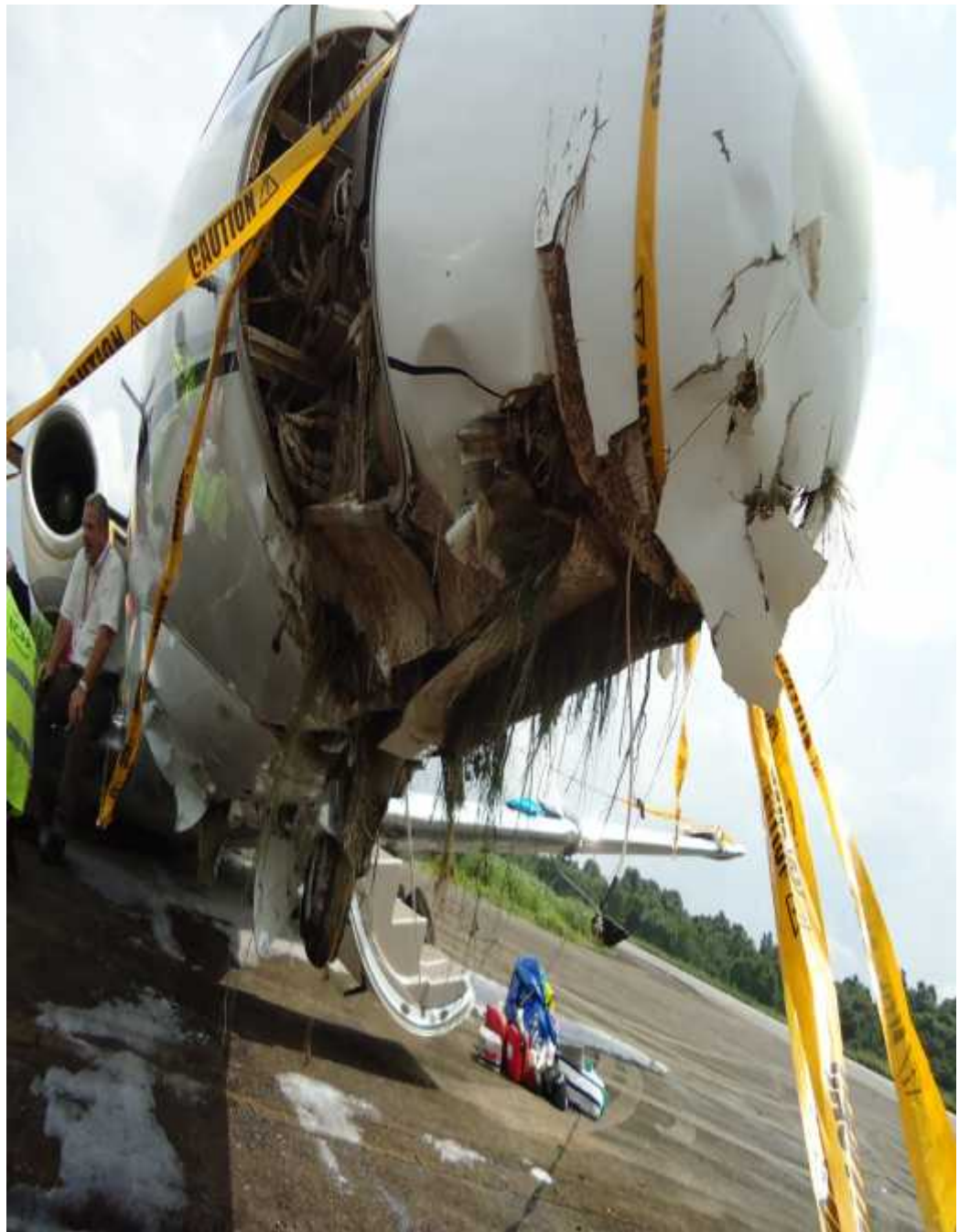
Fig 1.3c The damaged nose wheel and the Radome area
