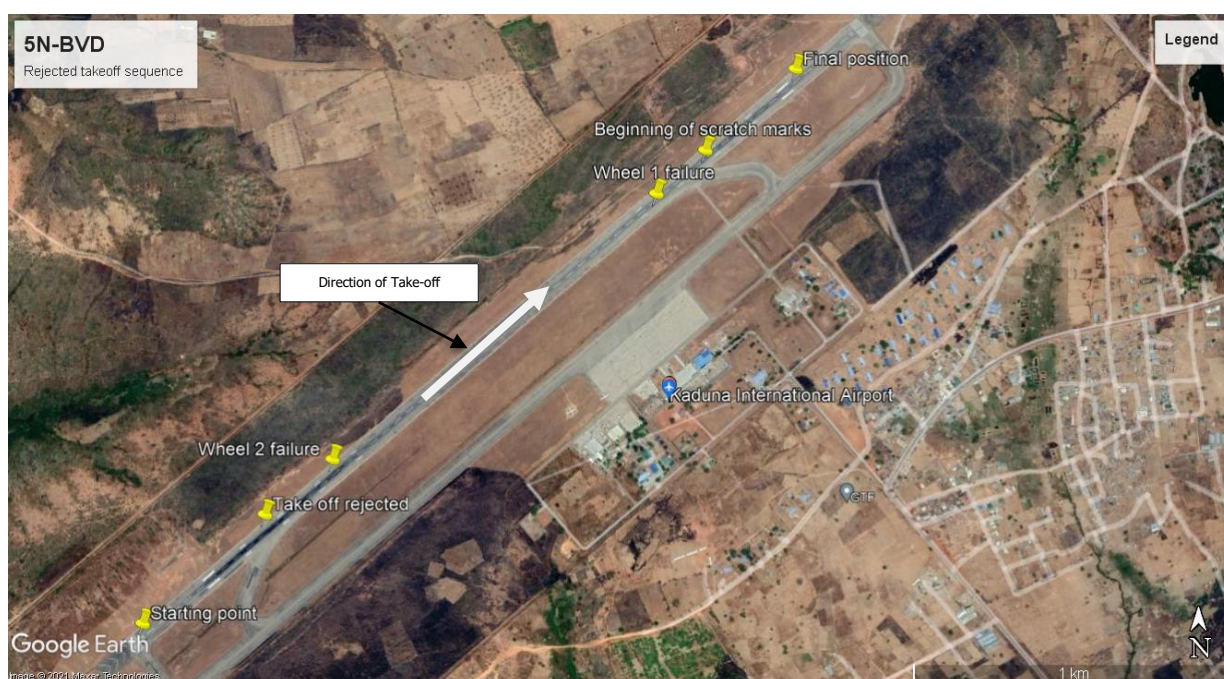
Figure 10: Sequence of events during the rejected take-off
