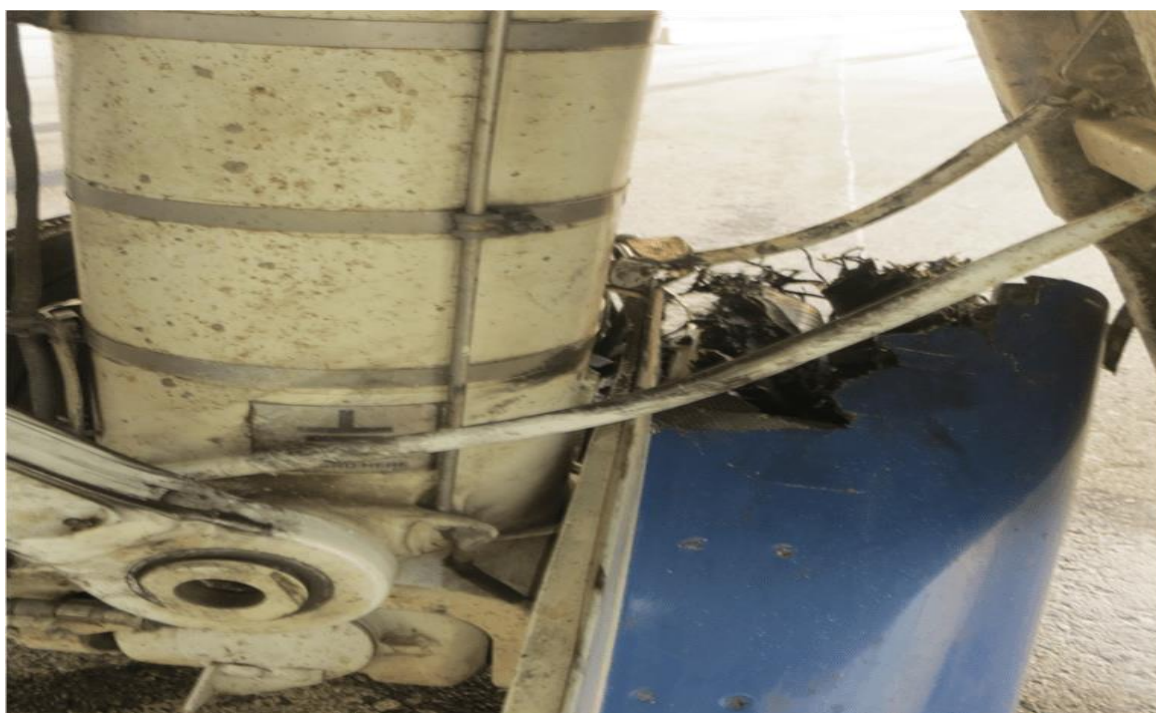
Figure 13: Torn left main landing gear door fairing
