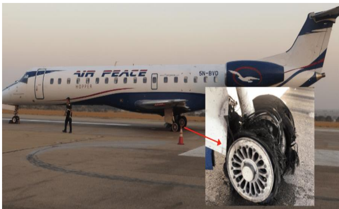
Figure 1: EMB-145 LR with registration marks 5N-BVD showing the condition of the No.1 main landing gear wheel assembly after the occurrence
