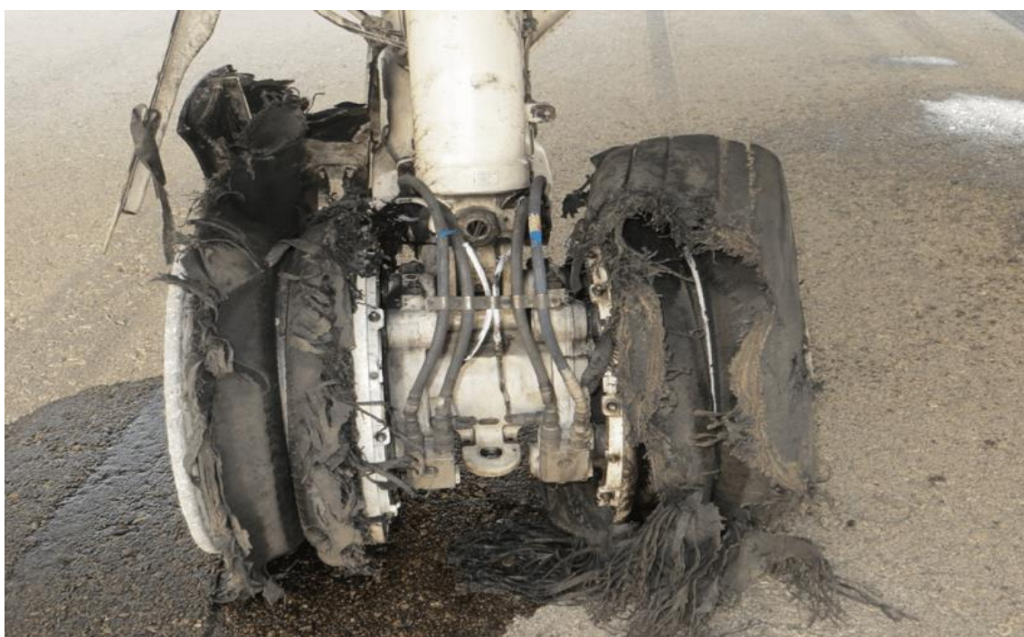
Figure 12: Damaged number 1 and 2 tyres with hydraulic leakage
