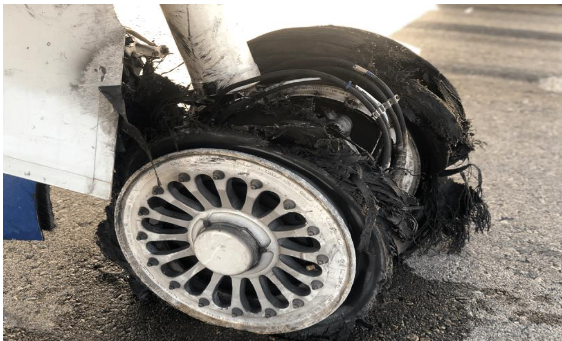
Figure 13: Torn left main landing gear door fairing
