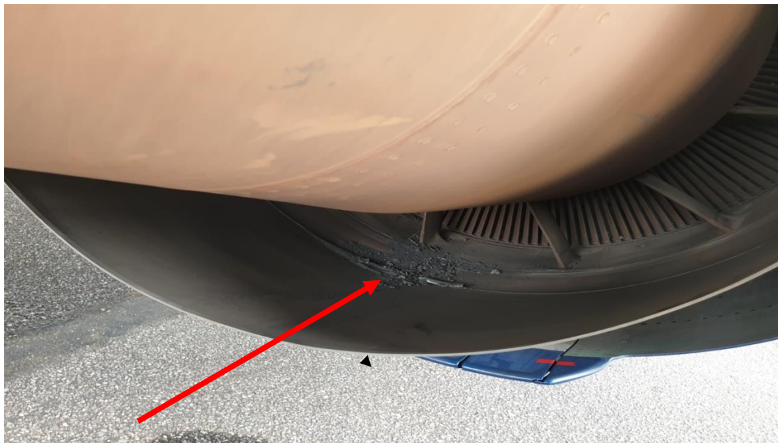
Figure 2: Photo of metal debris from the malfunctioned No. 2 engine
