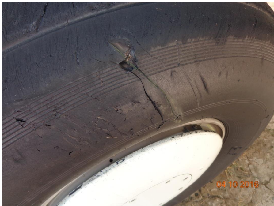
Figure 11: Photo of a deep cut on No. 4 main wheel tyre
