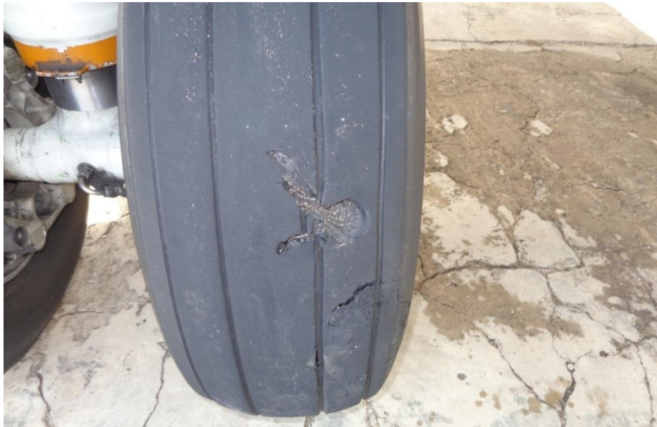
Figure 13: Photo of cuts and flat spots/abrasion on No. 2 main wheel tyre
