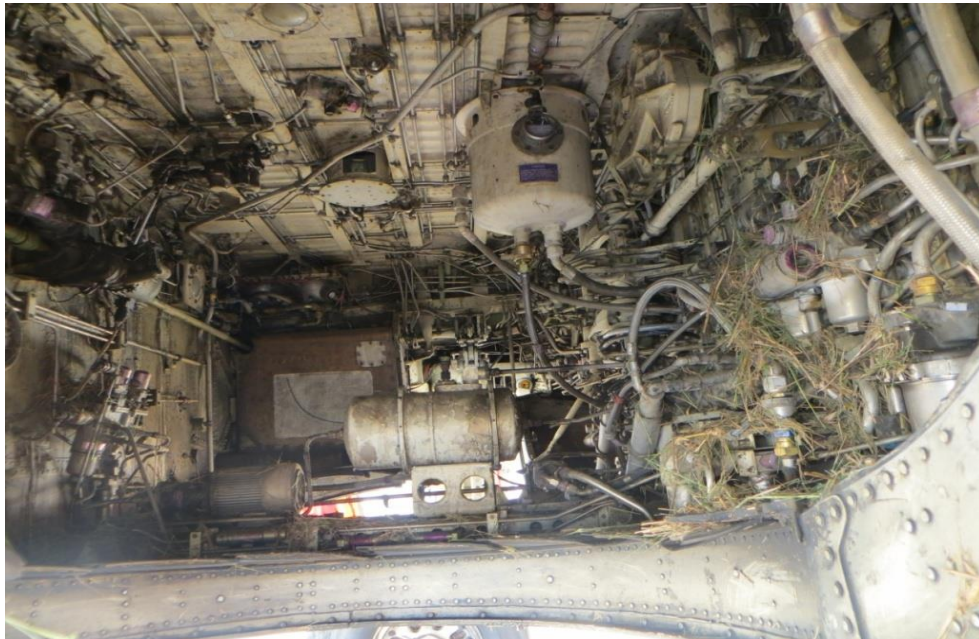
Figure 15: Photo of grass ingestion in the wheel well area
