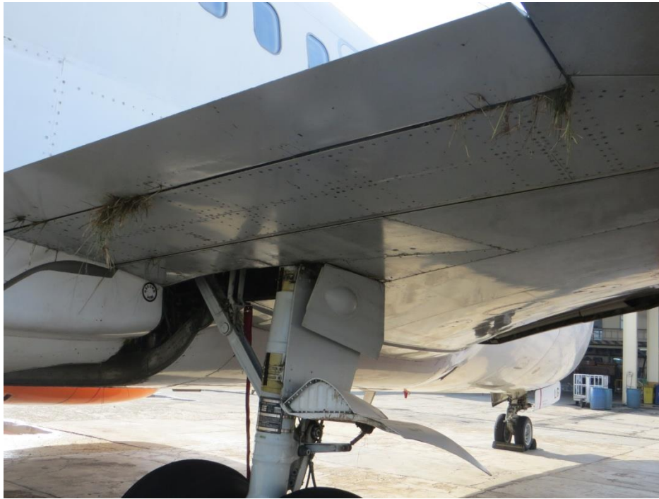
Figure 17: Photo of grass in the right inboard flap tracks
