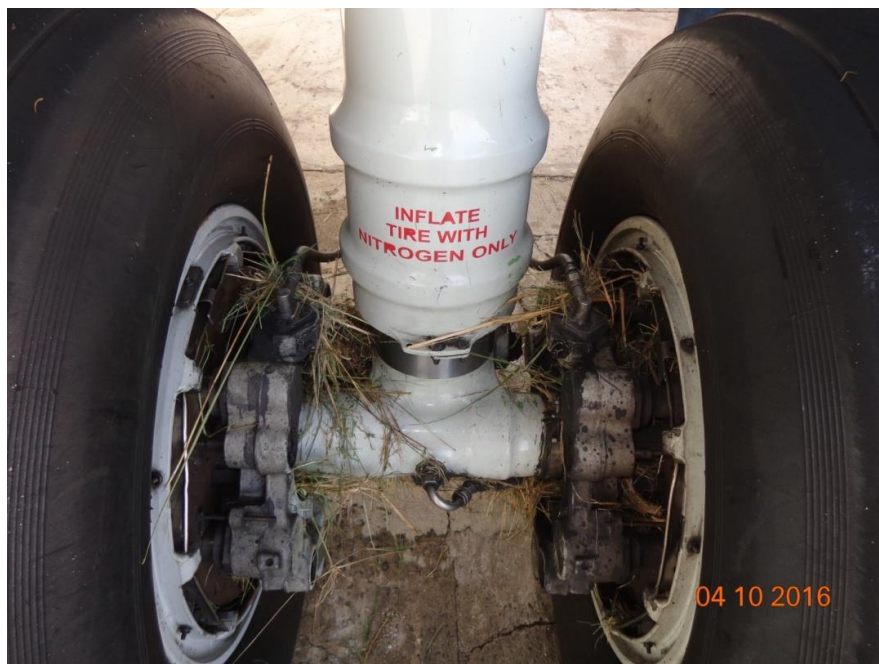
Figure 12: Photo of grass on right MLG assembly axle
