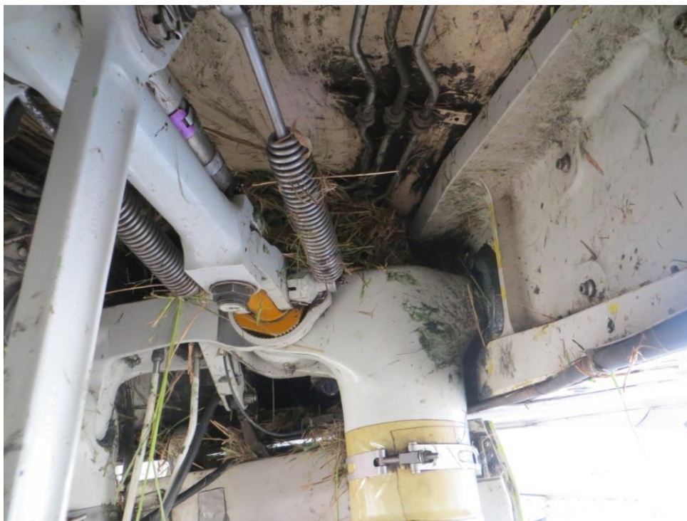
Figure 16: Photo of grass on right main landing gear attachment area
