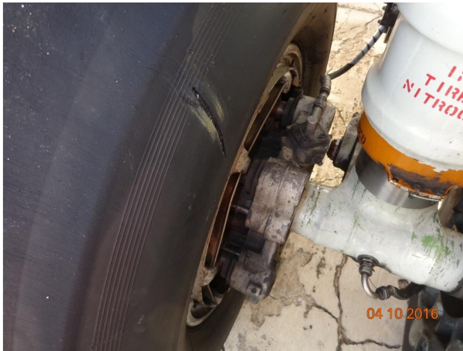
Figure 14: Photo of abrasion on No. 1 main wheel
