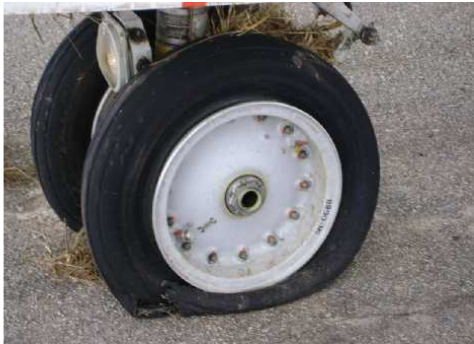
Fig 1.12c Picture showing nose landing gear with burst tires
