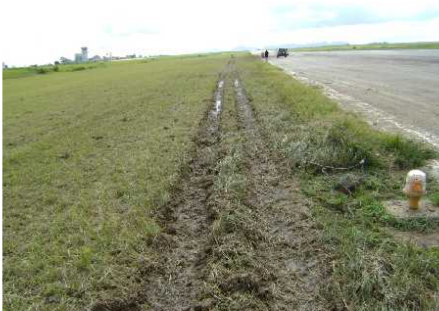
Fig 1.12f Picture showing tyre marks of aircraft veered off the runway 28
