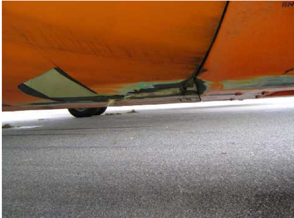
Fig 1.12d Picture showing under fuselage damaged
