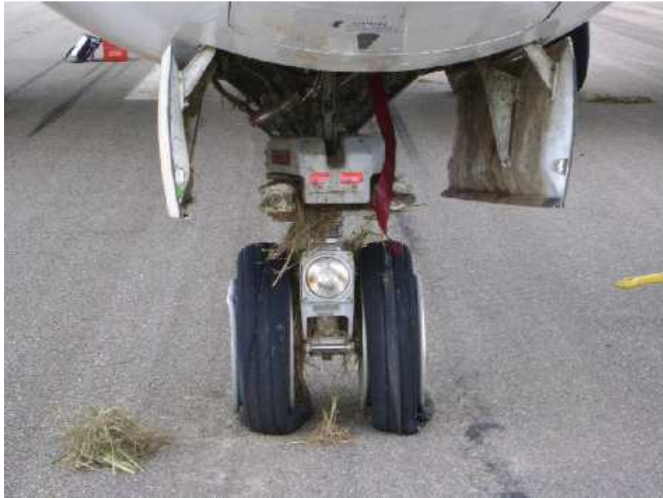
Fig 1.12b Picture depicting nose landing shock strut collapse with burst tires
