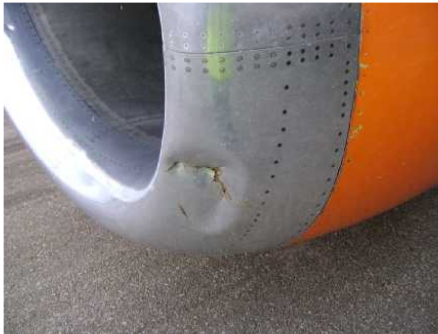
Fig 1.12a Picture showing damaged lower cowling
