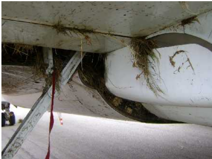
Fig 1.12e Picture showing engine cowling with ingested materials and lip damages
