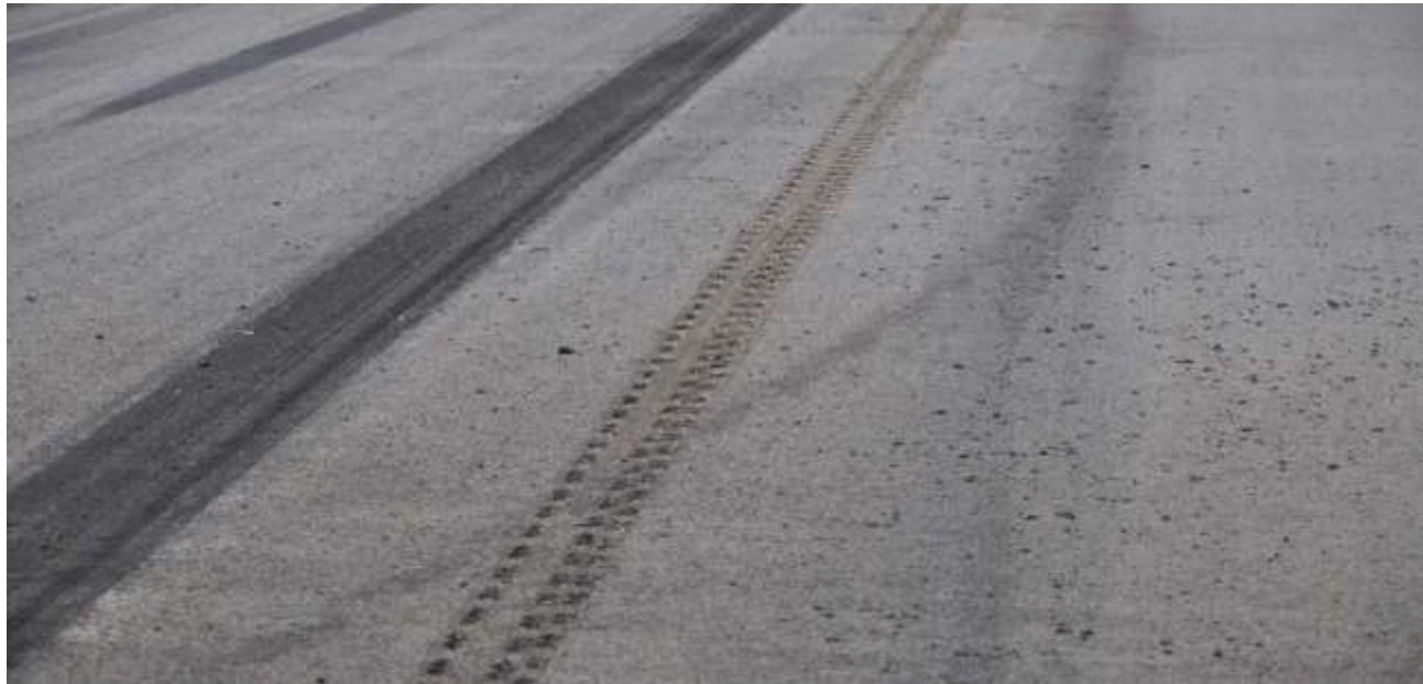
Figure 4: No. 1 Main brake assembly impact marks on the runway
