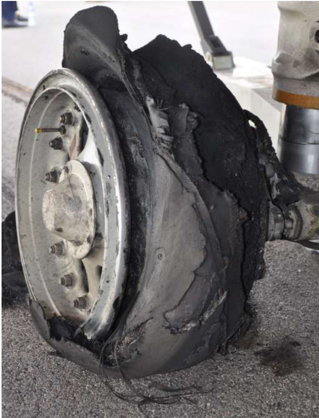
Figure 6: Damaged No. 2 main wheel assembly
