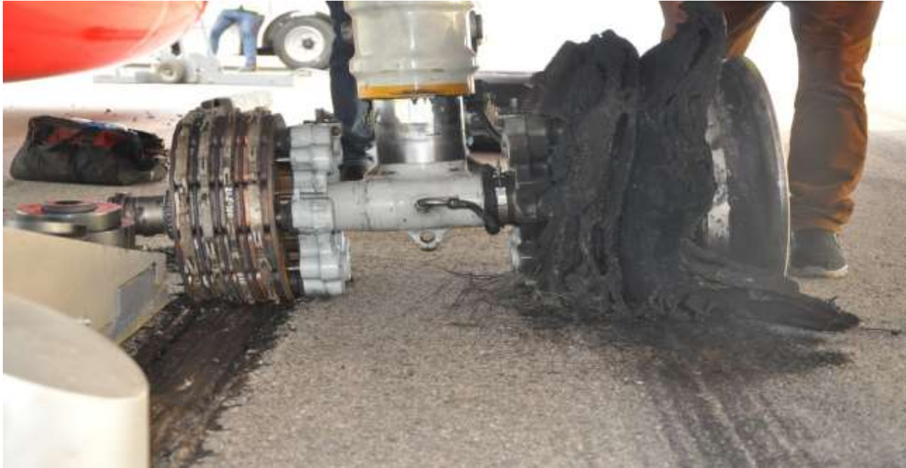
Figure 2: Damage to the No. 1 main landing gear wheels of 5N-MBD
