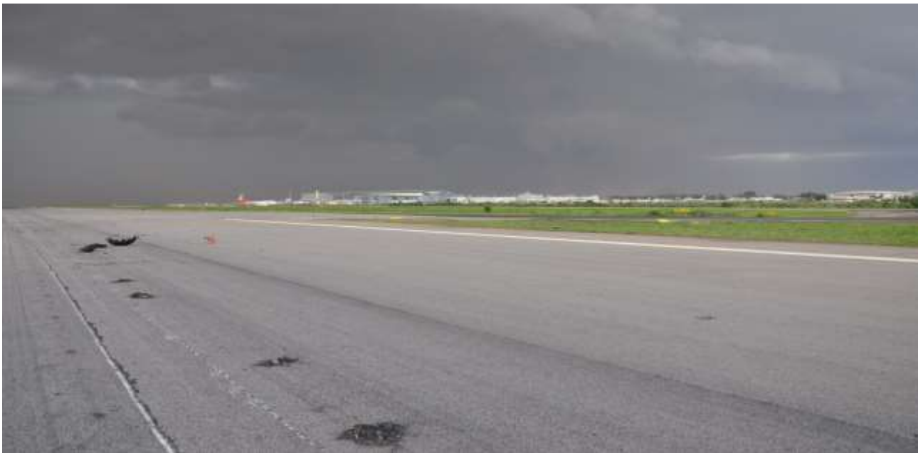
Figure 3: Debris of No. 2 main wheel tyre with No.2 wheel impact marks on the runway.
