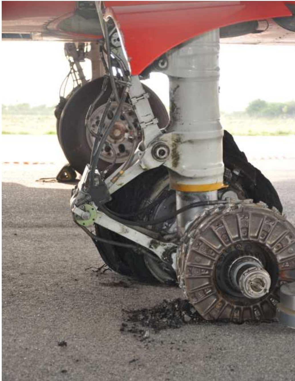
Figure 7: No.1 brake assembly with the roller bearings after the wheel fell off
