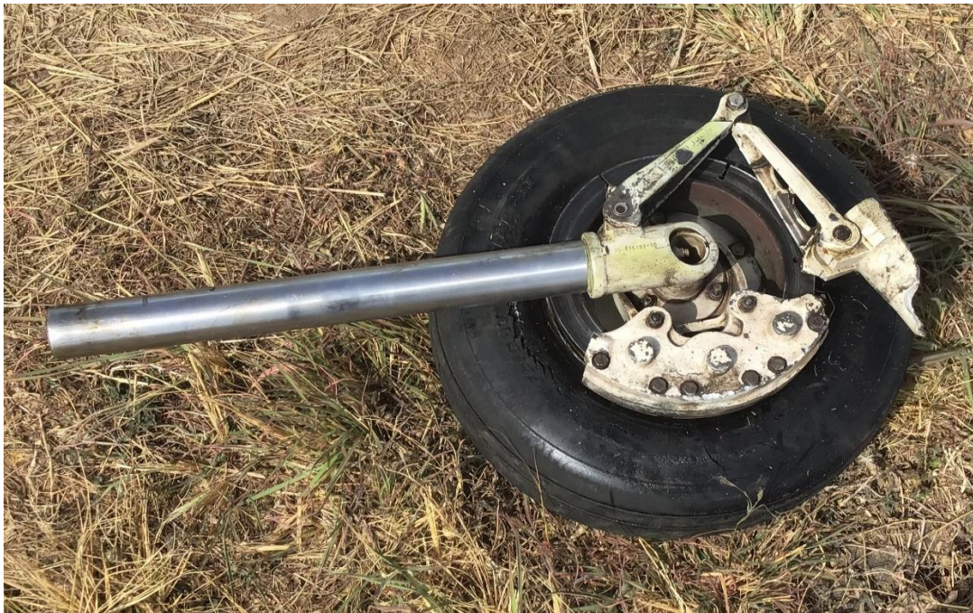
Figure 4: The sheared right main landing gear
