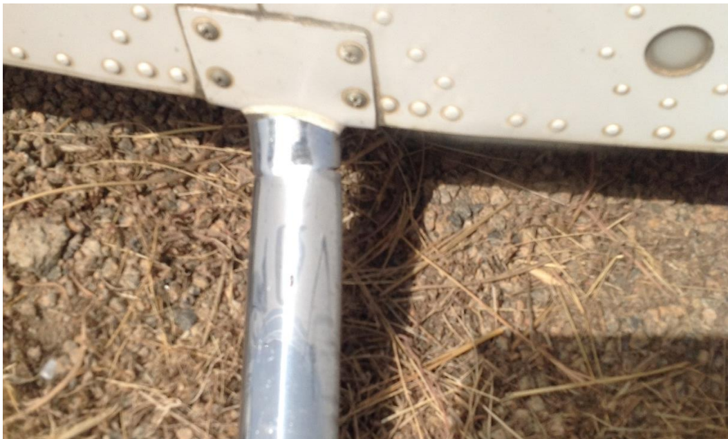
Figure 8: The broken step
