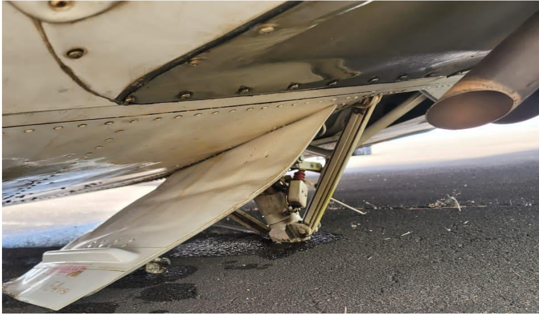
Figure 5: The remaining part of the landing gear attach to the aircraft
