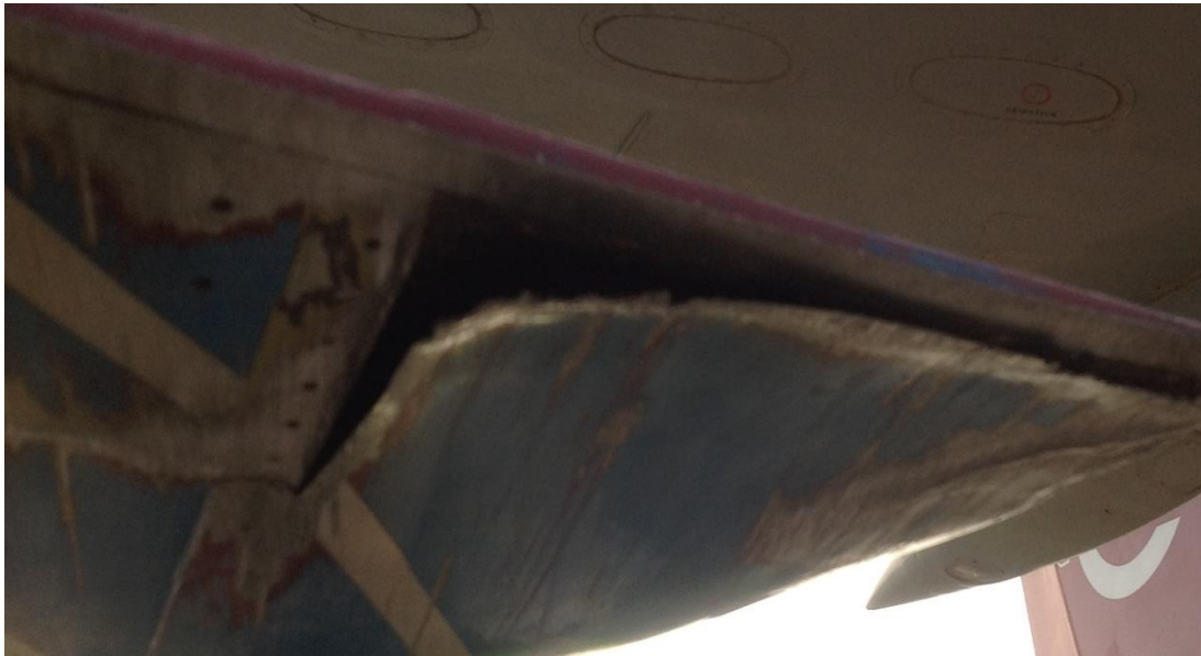
Figure 9: The torn right tank from the bottom
