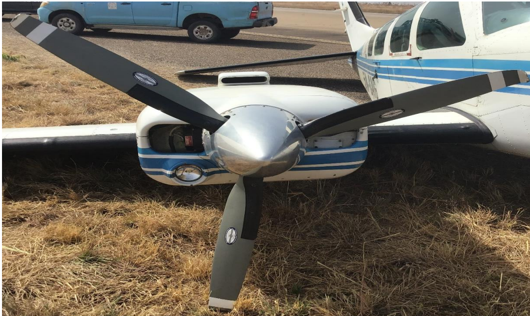
Figure 7: Bent propeller blade at the tip
