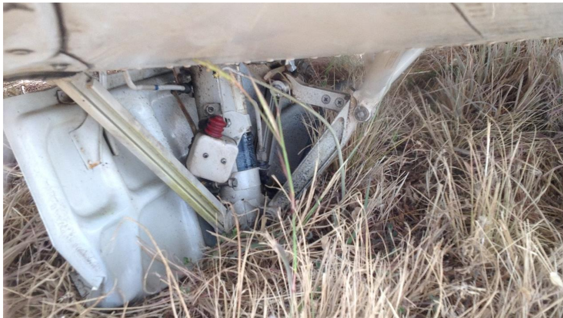
Figure 6: The remaining part of the landing gear attach to the aircraft
