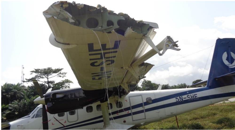
The damaged left Wing of 5N-SHE
