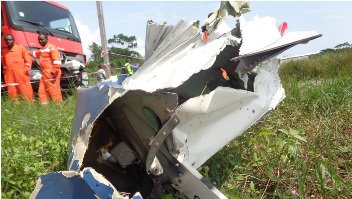
Picture of debris from damaged left Wing Tip assembly of the aircraft
