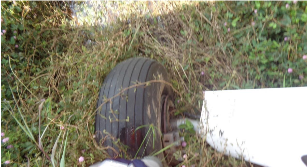
Right Main Wheel stuck in grassy-mud
