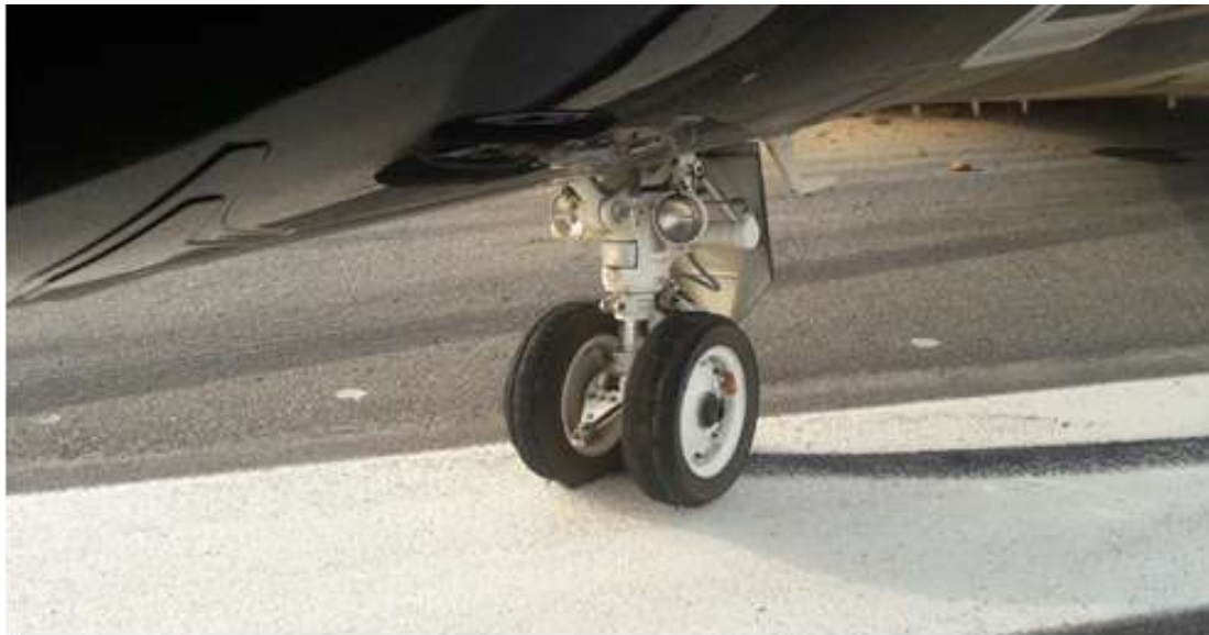
Figure 5: Picture showing the damaged nose wheel tyre
