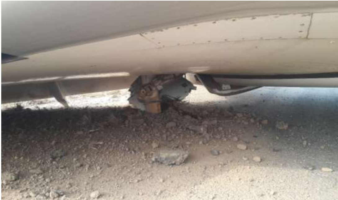
Figure 3: Picture showing right main landing gear detachment point at the under carriage
