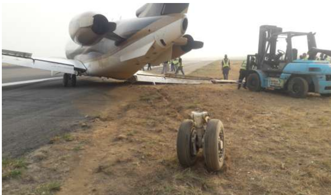
Figure 2: Picture showing detached right main landing gear
