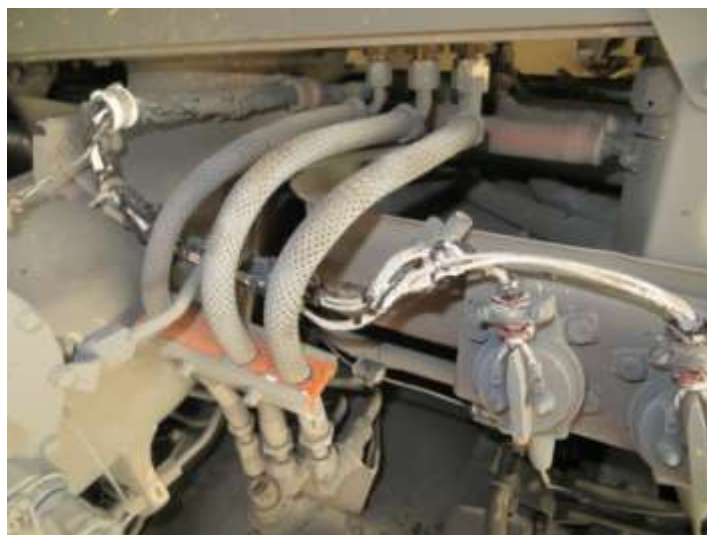
Figure 2: Charred wires within the engine cowling
