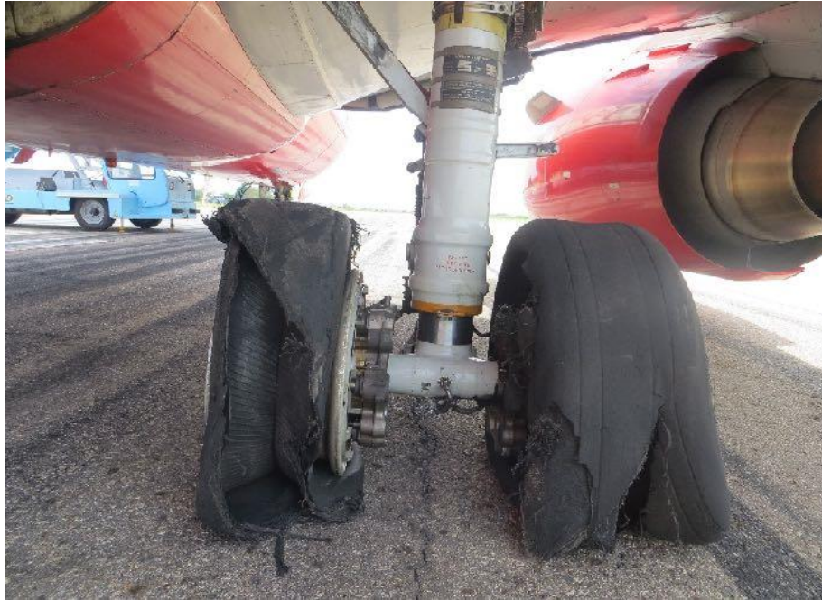
Figure 9: Failed Tyres Number 3 and Number 4
