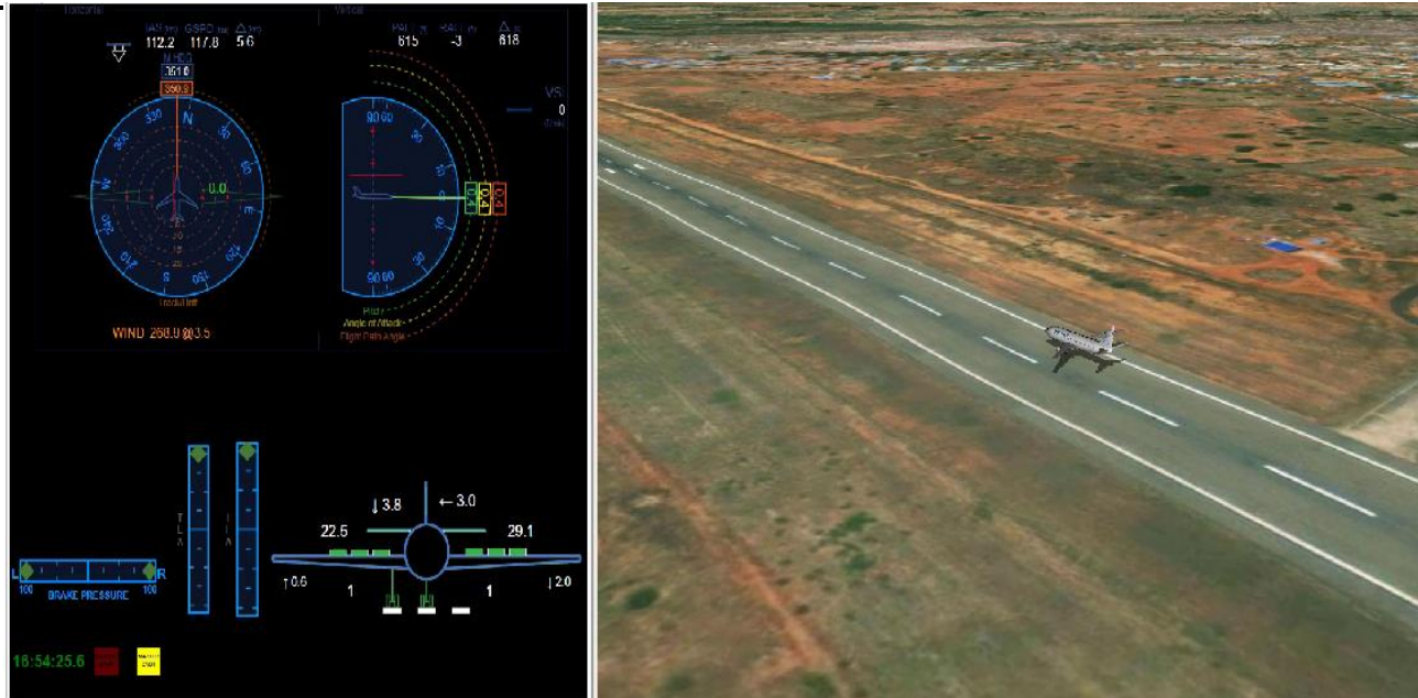
Figure 15: Deployment of reversers, brakes and speed brakes
