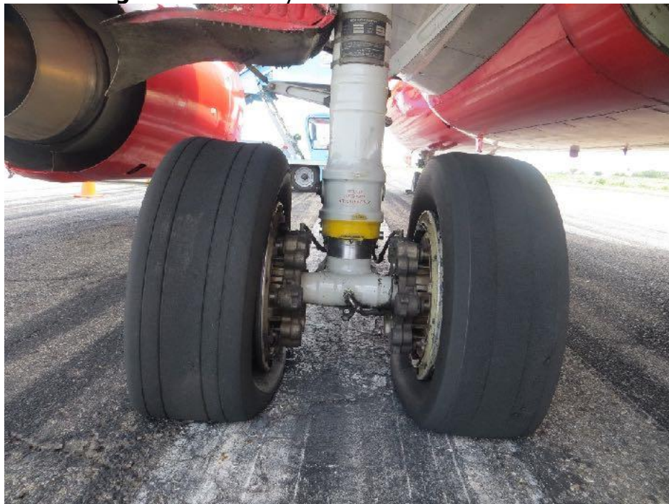
Figure 9: Failed Tyres Number 3 and Number 4
