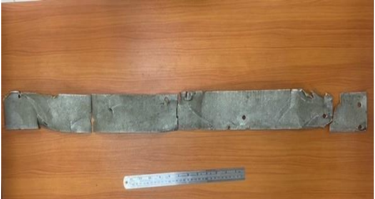
Figure 3: Foreign Object Debris recovered from the runway (ruler to show scale)
