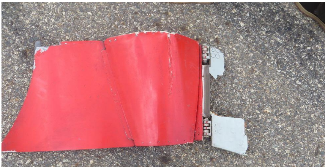
Figure 11: Torn section of Right MLG shock strut door
