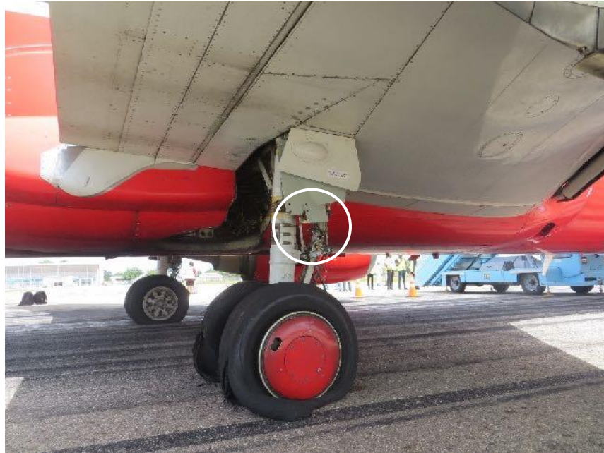
Figure 11: Torn section of Right MLG shock strut door
