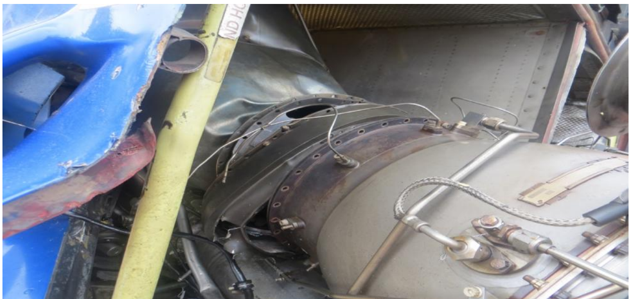
Fig. 10 Engine No. 2 suffered an uncontained failure.
