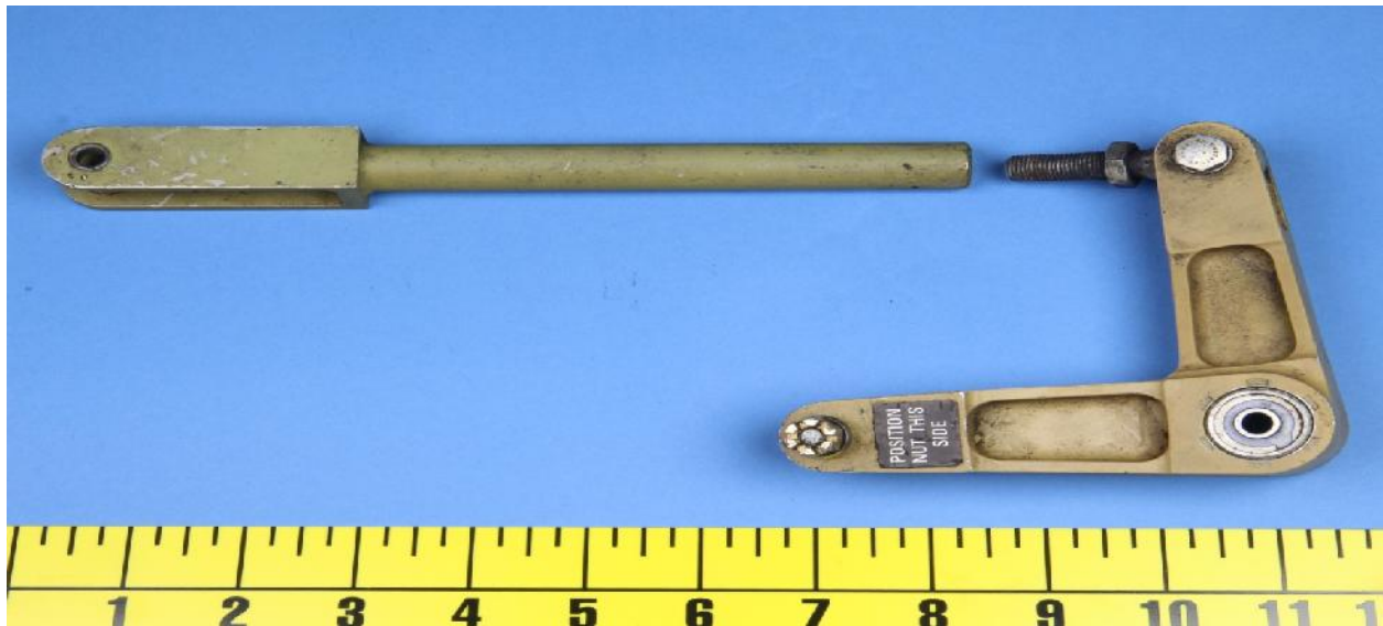
Fig. 8 Control Pushrod and Control Rod end with bearing and Jamnut
