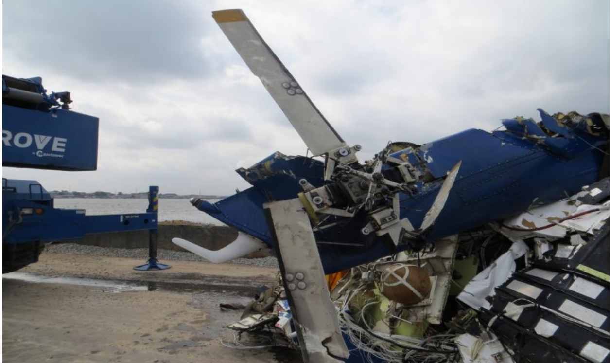
Fig. 2 Part of the destroyed tail Rotor area.
