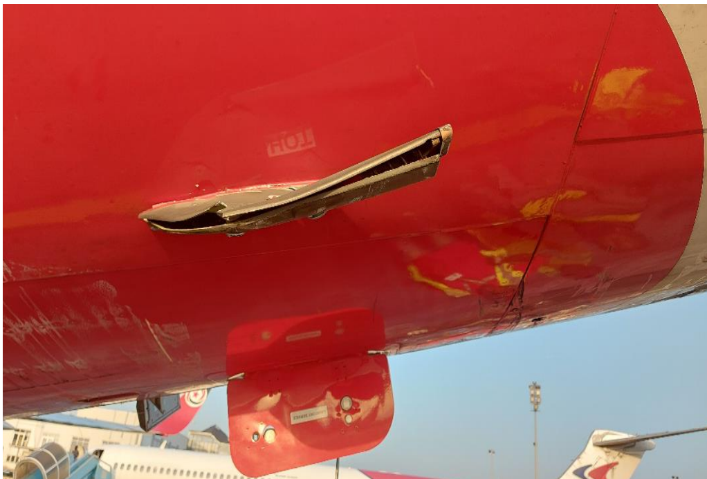
Figure 3: Dent around the rear pressure bulkhead area
