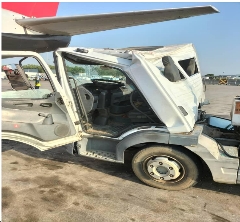
Figure 7: Damaged lavatory service truck after the incident
