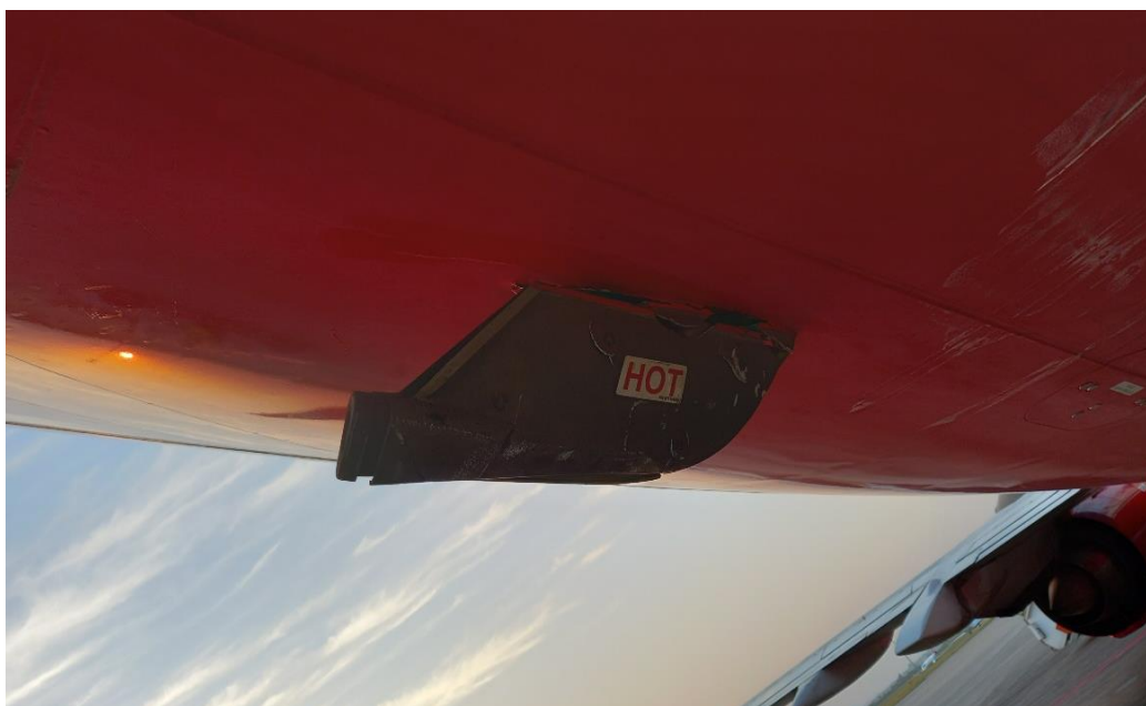
Figure 4: damaged rear galley drain mast
