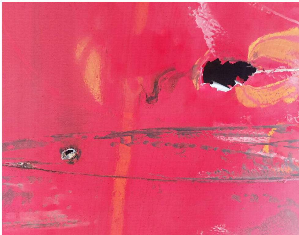
Figure 5: Three holes on the aft of the fuselage unpressurized area
