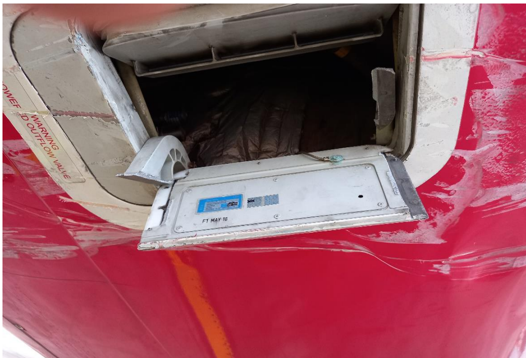
Figure 6: Broken outflow valve
