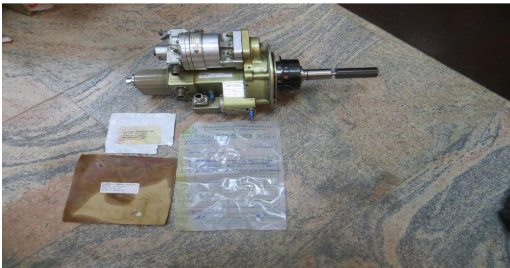
Figure 9: Photo showing the defective left engine PCU
