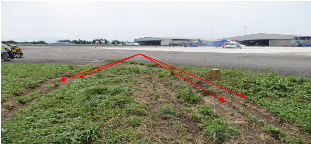
Figure 7: Photo showing the aircraft's tyre marks on the grass
