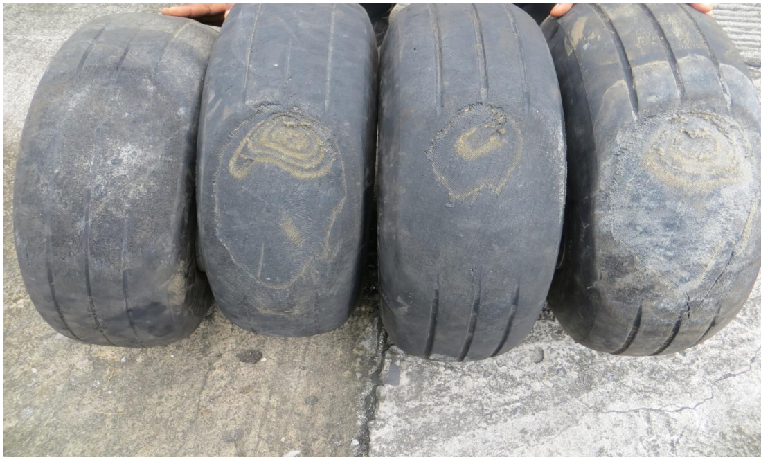
Figure 1: Photo showing the aircraft's flat spotted main wheel tyres
