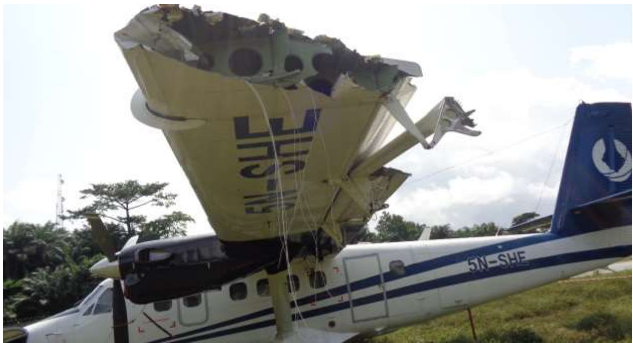
Figure 6: Damaged left wing of 5N-SHE
