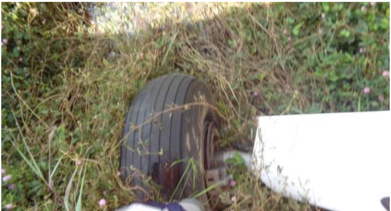
Figure 8: The right main wheel stuck in grass-verge
