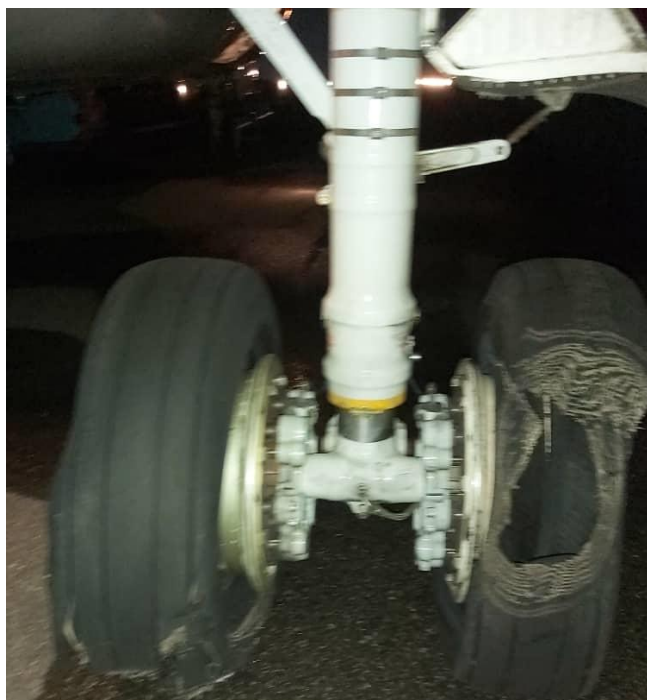
Figure 7: Rear view of damaged no. 3 & 4 main wheel tyres
