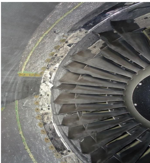
Figure 5: Damaged fan blades of number 1 engine caused by ingestion of debris from the burst tyre
