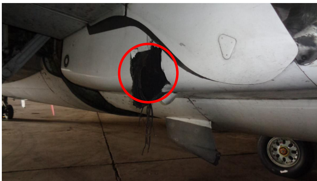
Figure 8: Tyre debris stuck in the flap track fairing
