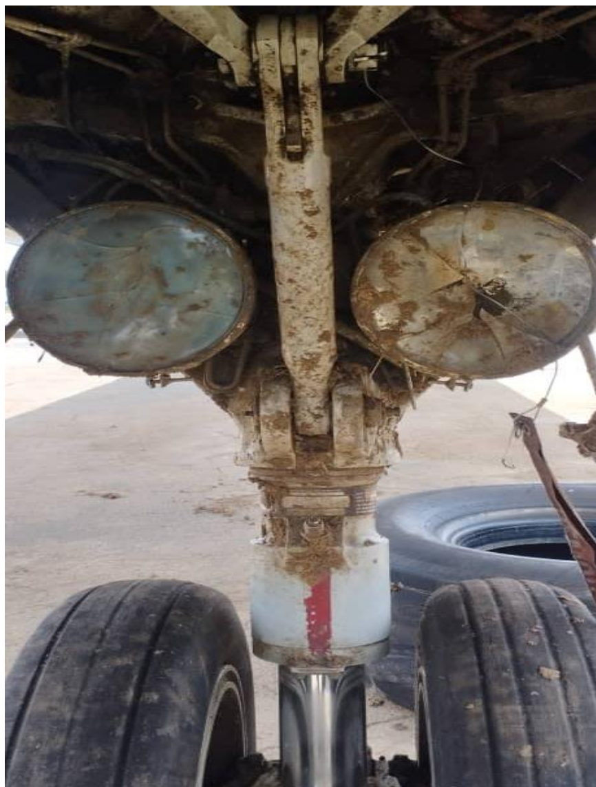
Figure 4: Damaged nose landing gear light
