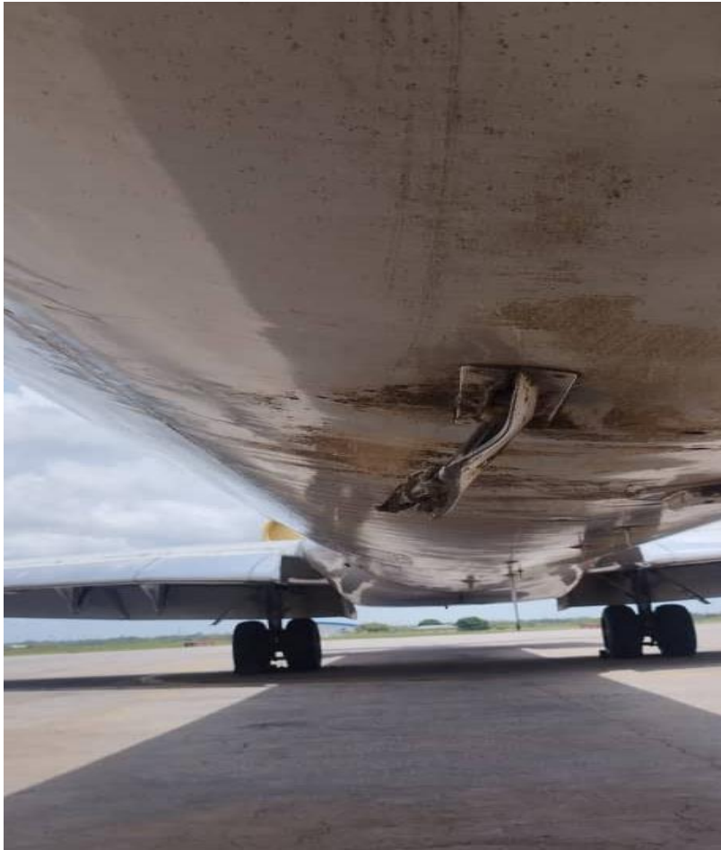
Figure 3: Damaged Galley Drain & Antenna
