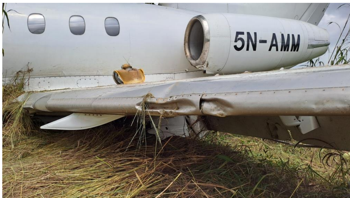
Figure 7: Close-up of damage to the left wing leading edge
