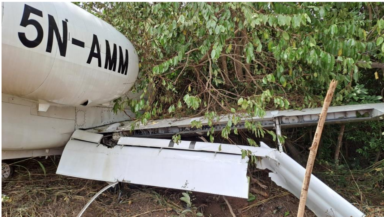
Figure 5: Damage to the right wing flaps
