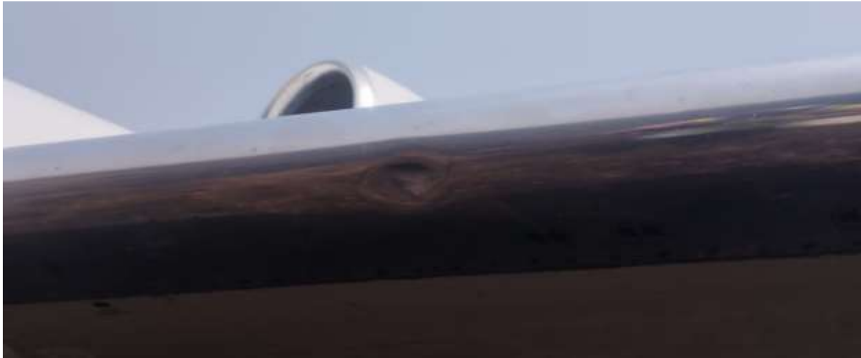
Figure 8: Dent created about the mid-section of left wing leading edge surface
