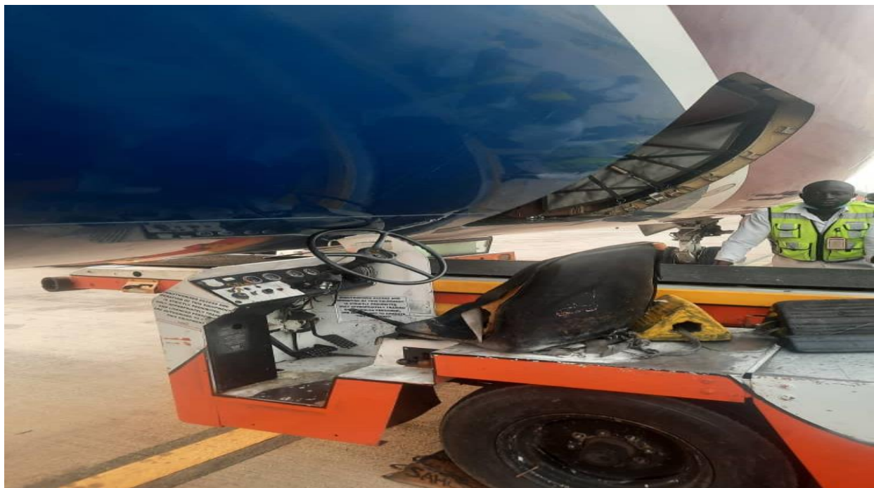
Figure 2: The conveyor belt truck still under the aircraft after the occurrence (Picture taken by the crew)
