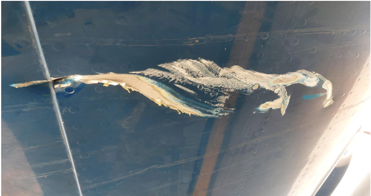
Figure 3: Puncture to the fuselage of the Arik air aircraft (a pressurised section of the aircraft)
