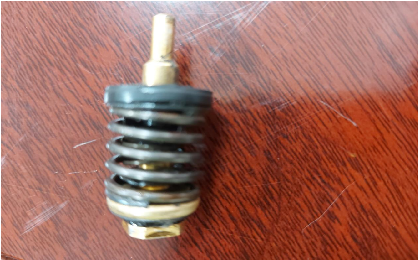
Figure 7: Brake proportioning valve of the truck where the leakage was traced to
