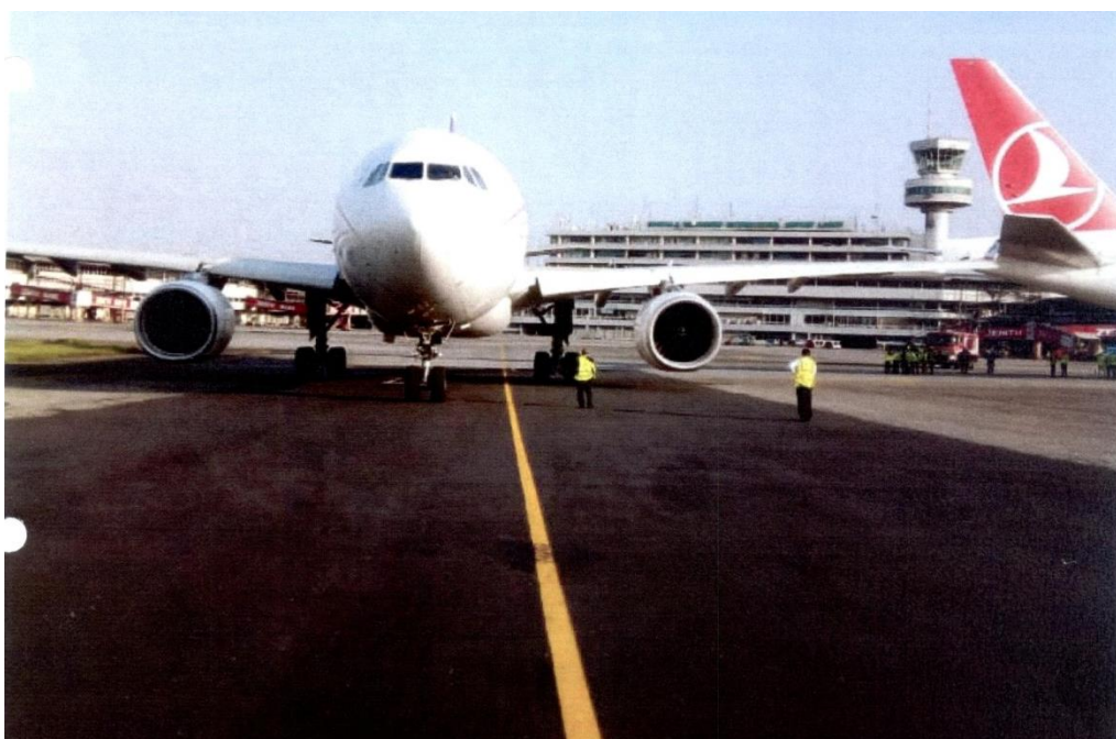
Figure 6: The deviation of MEA572 airlines aircraft from the taxi line
