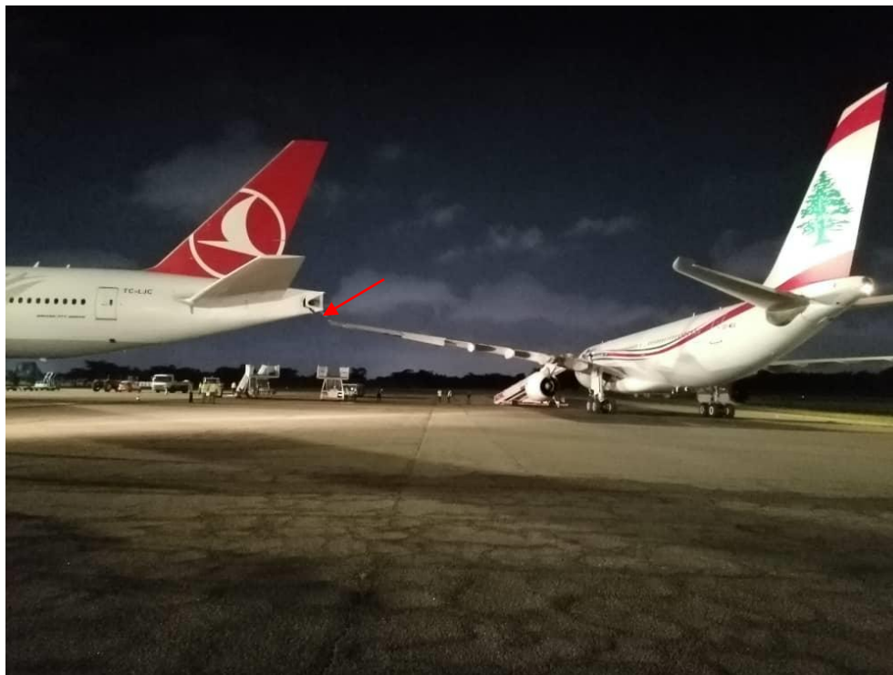
Figure 3: MEA572 aircraft winglet clipped the APU exhaust of the Turkish aircraft
