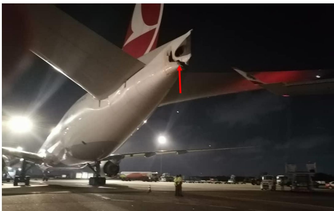
Figure 4: Damaged APU exhaust area of the Turkish Airlines aircraft
